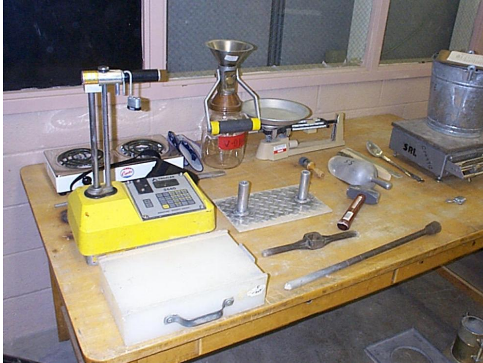
Fig. 1.2 Equipment for Field Moisture and Density Testing
