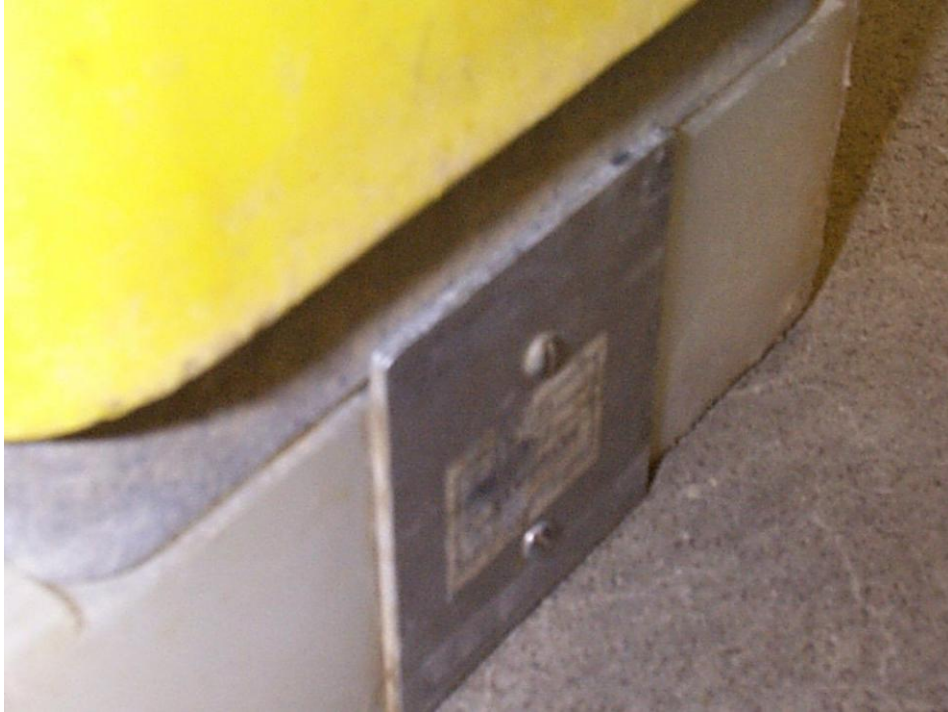
Fig. 1.8 Nuclear Gauge on Calibration Block
