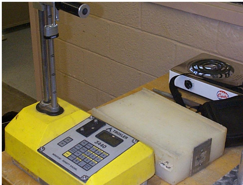
Fig. 1.5 Nuclear Gauge Calibration Block
