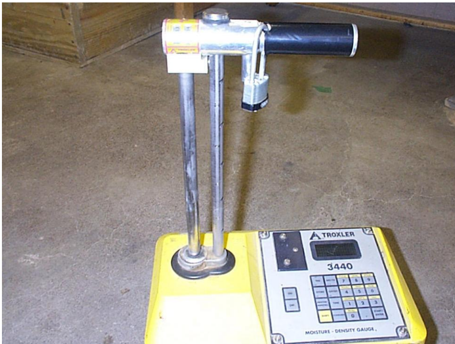
Fig. 1.9 Nuclear Gauge Locked for Safety when Not in Use
