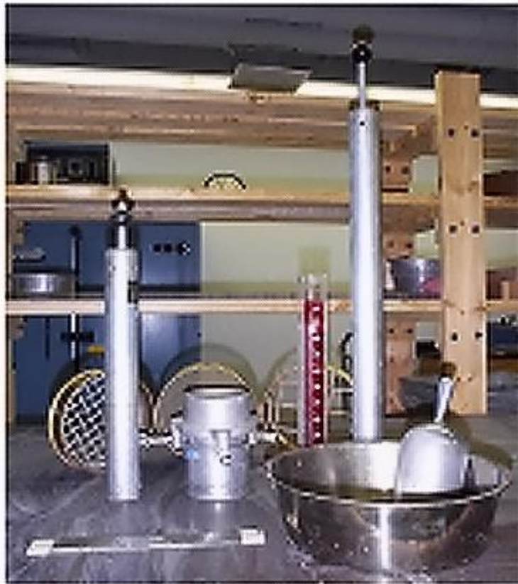
Figure 1.11 Apparatus for T 99 and T 180
