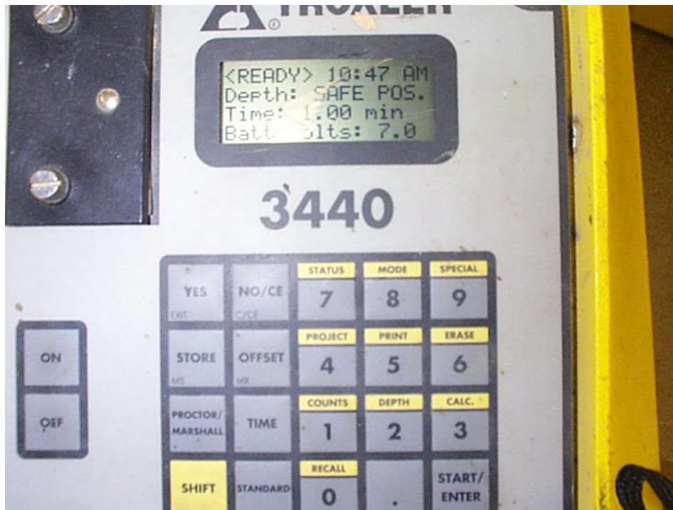
Fig. 1.4 Nuclear Moisture – Density Gauge Display Panel
