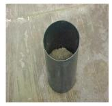
Strength Test Specimens Strike off excess concrete from the surface with a tamping rod and float or trowel as required. Use a minimum amount of manipulation necessary to produce a flat, even surface.
