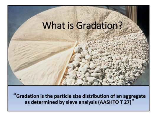
A complete well graded concrete utilizes the cement paste more efficiently & will decrease shrinkage while improving workability and provide slightly higher slump without additional water.
