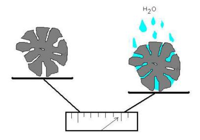
Figure 14. Increase in mass due to absorption of water The formulas for the above-mentioned determinations are as follows:
