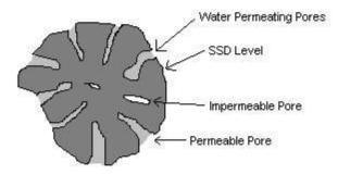
Figure 12 - Diagram of Bulk SSD. Specific Gravity SSD mass is the Saturated Surface Dry Condition and includes the mass of the water in the permeable pore space.
