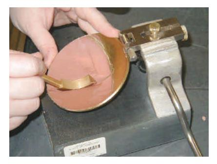
Figure 7 - Grooving the Soil Specimen
