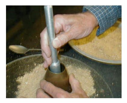
Figure 3 - Tamping sample using the Cone Method to determine SSD
