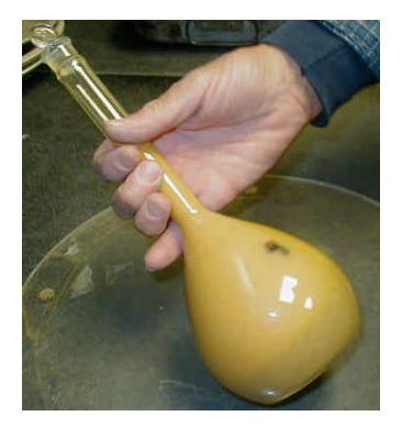
Figure 6 - Rolling of pycnometer
