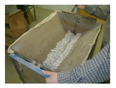
Figure 5 - Sample spread uniformly in splitter
