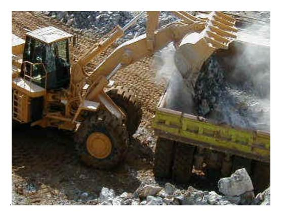
Fig 4.3 Front end loader loading off road vehicle from muck pile.
