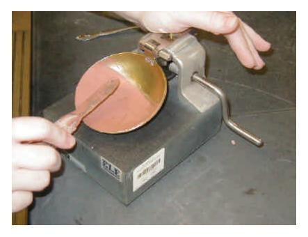
Figure 6 - Spreading Specimen in Liquid Limit Cup
