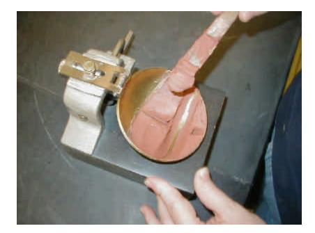
Figure 9 - Removing the Moisture Content Specimen
