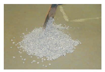
Figure 9 - Improper mixing of sample for quartering
