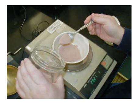
Figure 2 - Weighing Material for Test Specimen
