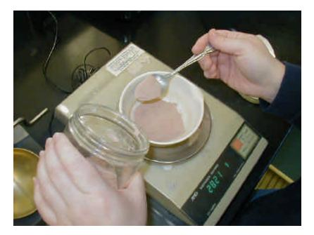
Figure 4 - Weighing Test Specimen
