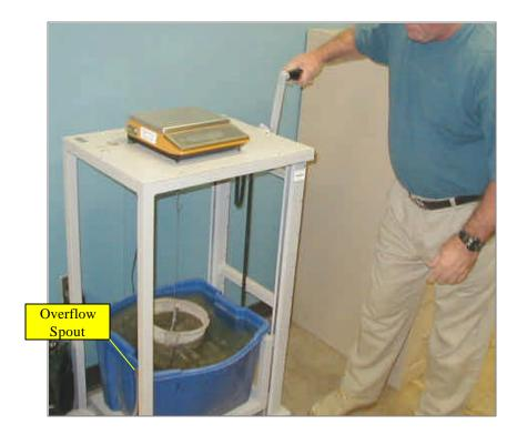
Figure 2 - Coarse Aggregate Gravity Apparatus.
