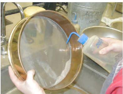
Figure 5 - Material retained on the 75 µm (No. 200) sieve after washing
