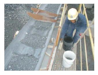
Figure 4 - Three belt cuts to make one sample.
