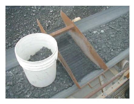
Figure 2 - Belt Cut Using Template
