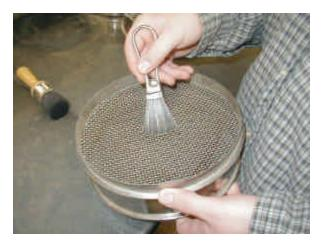
Figure 3 - Use Wire Brush on Coarse Sieves
