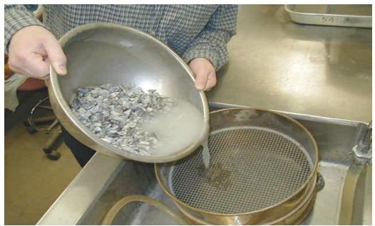
Figure 3 - Fines suspended in the water are washed over a 2.36 mm (No. 8) or 1.18 mm (No. 16) and a 75 µm (No. 200) sieve.
