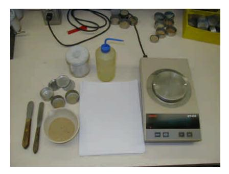
Figure 1 - Equipment for Plastic Limit
