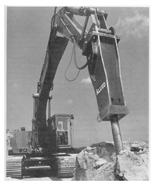
Fig 4.8 Backhoe mounted hydraulic impact hammer.
