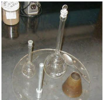
Figure 1 - Pycnometers, mold & tamper
