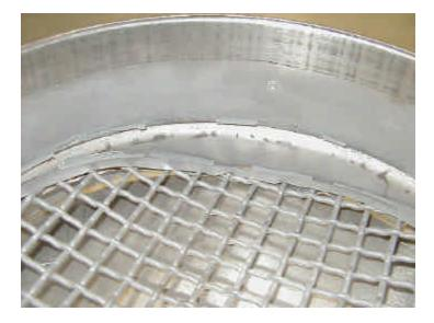
Figure 5 - Cracked Outer Seam
