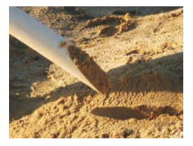
Figure 1 - Stockpile sampling with a sampling tube
