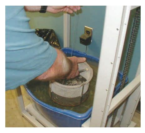
Figure 4 - Water tank: large enough to completely immerse basket containing aggregate and equipped with an overflow valve to keep water at a constant level.
