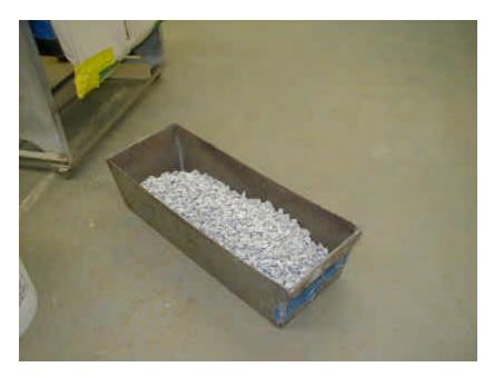
Figure 7 - Proper sized pan to fit splitter
