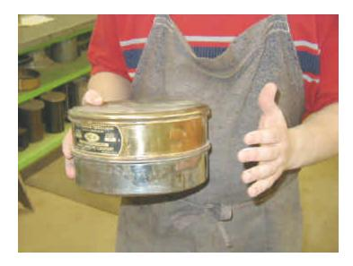
Figure 6 - Checking thoroughness of sieving
