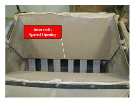
Figure 8 – Incorrect Openings
