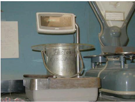
Figure 2 - 1/10 cubic foot measure.
