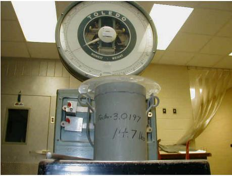
Figure 1 - 1/3 cubic foot measure.
