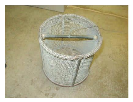
Figure 3 - Sample container: wire basket of 3.35 mm (No. 6) or less mesh wire cloth, with a capacity to contain aggregate with a nominal maximum size of 37.5 mm (1½ in.) or smaller.
