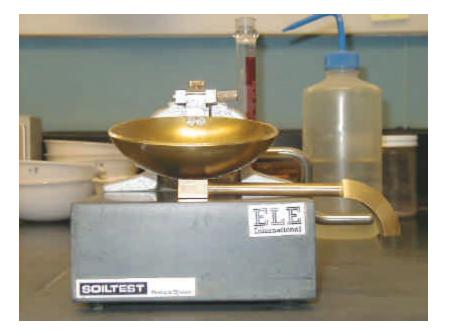
Figure 3 - Checking Contacts with Height Gage
