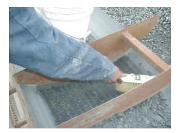
Figure 3 - Cleaning fines from belt.
