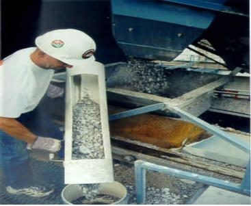
Figure 1 - Streamflow Sampling
