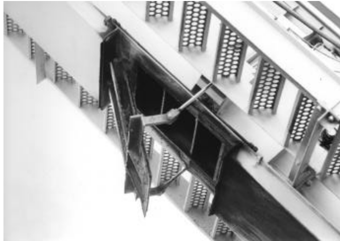
Figure 11.9 Drop-out chute in slat conveyor.
