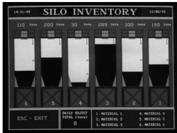
Figure 11.5 Modern silo control screen showing silo inventory.
