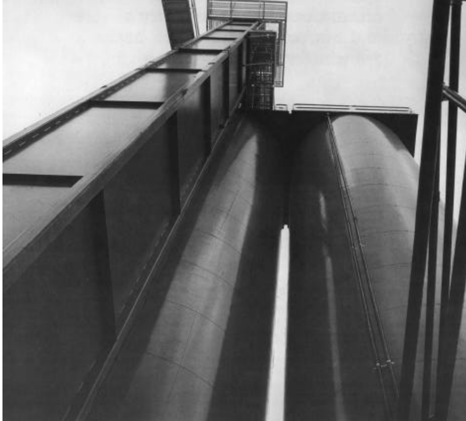
Figure 11.6 Bucket elevator feeding storage silos on hot mix plant.
