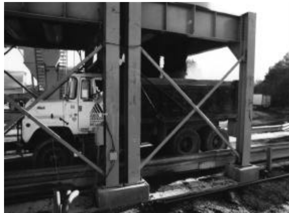
Figure 11.25 Truck being loaded from silo on truck scale.
