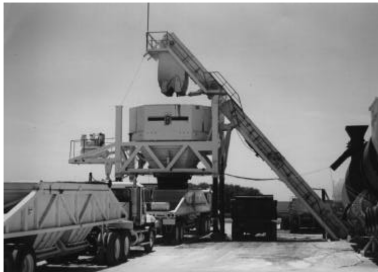
Figure 11.29 Portable, self-erect, reverse weigh silo.
