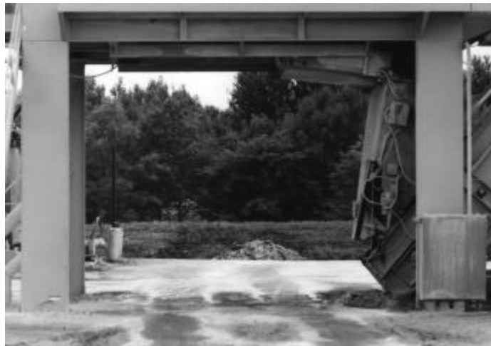
Figure 11.11 Knuckle chute in stored position.
