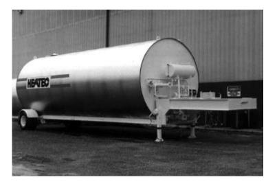
Figure 4.12 Portable, direct fired, asphalt tank.
