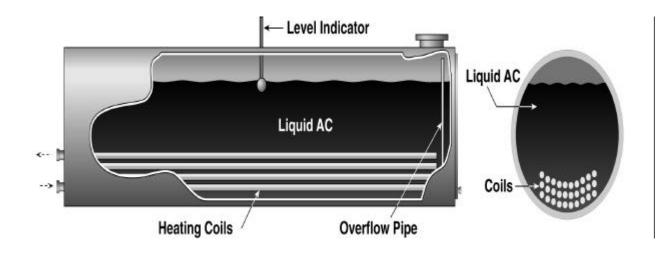
Figure 4.1 Typical horizontal asphalt tank.
