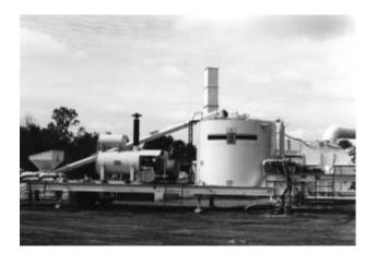
Figure 4.15 Crumb rubber modified asphalt processing system and tanks.
