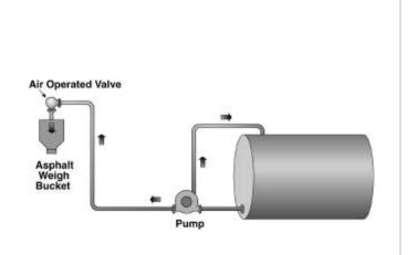
Figure 4.24 Asphalt fill valve on batch tower.
