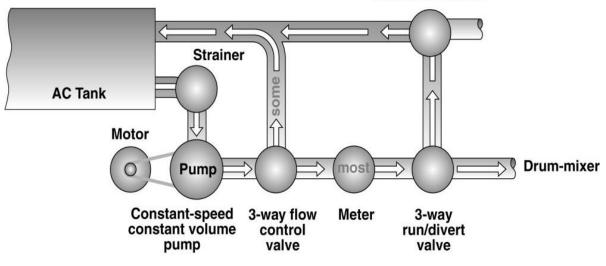
Figure 4.25 Asphalt metering system for drum-mixer plants with constant speed constant volume pump and flow control valve.
