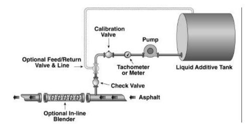
Figure 4.28 Typical asphalt additive tank system.
