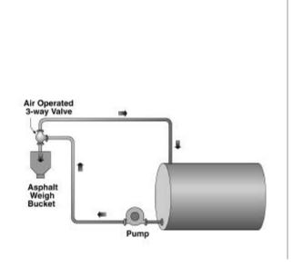
Figure 4.23 Two line asphalt system for batch tower.
