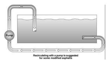
Figure 4.14 Recirculating with a pump is suggested for some modified asphalts.
