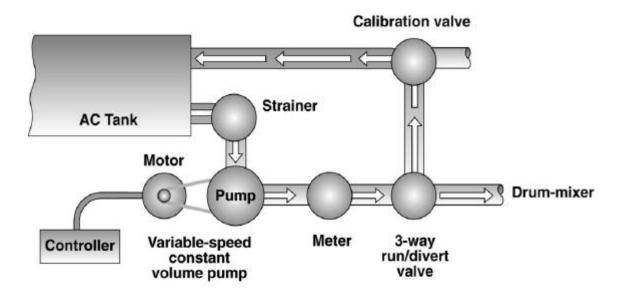
Figure 4.27 Asphalt metering system for drum-mixer plants with variable speed, constant volume pump.
