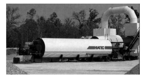
Figure 4.3 Portable asphalt tank.
