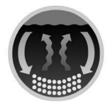
Figure 4.13 Natural convective currents in an asphalt storage tank.
