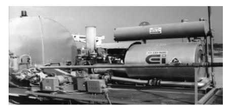
Figure 4.6 Hot oil heater to heat asphalt tanks.
