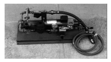
Figure 4.29 Typical liquid additive pumping skid including pump/motor and tachometer.
