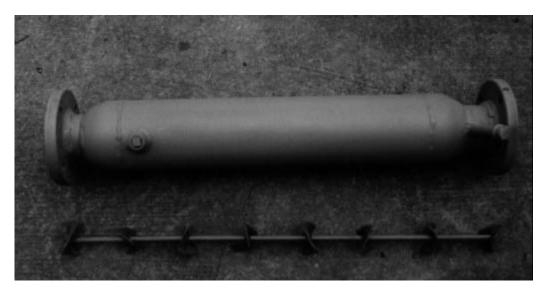
Figure 4.32 Liquid additive static in-line blender.
