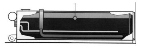
Figure 4.11 Typical direct fired asphalt tank.
