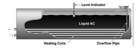
Figure 4.18 Safety overflow pipe in AC tank.
