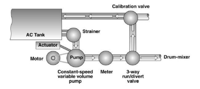
Figure 4.26 Asphalt metering system for drum-mixer plants with constant speed variable volume pump.
