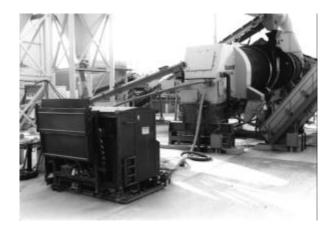
Figure 4.16 Fiber adding system with tank.
