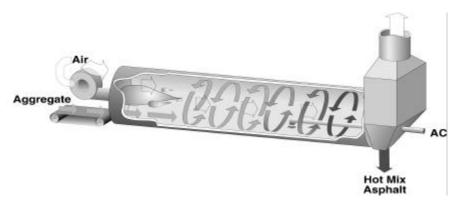
Figure 5.3 Typical parallel-flow drum-mixer.
