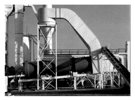
Figure 5.2 Counter-flow dryer on batch plant.
