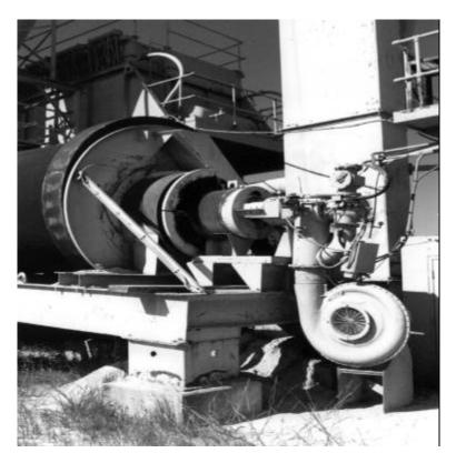
Figure 5.25 Older burner with combustion chamber.
