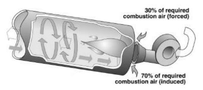
Figure 5.20 Induced draft burner.
