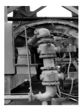
Figure 5.55 Rotary elevator discharge.
