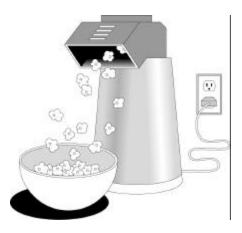
Figure 5.11 Example of convective heat transfer.
