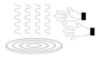
Figure 5.12 Example of radiant heat transfer.
