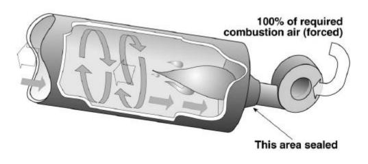
Figure 5.22 Total air burner.
