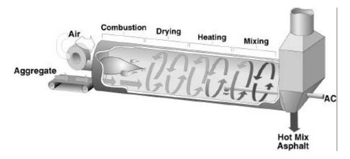
Figure 5.8 Parallel-flow drum-mixer zones.
