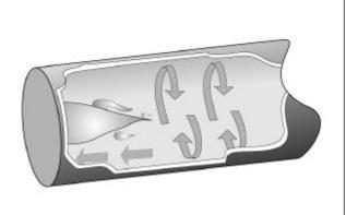
Figure 5.36 Gravity aids movement of aggregate through dryer.
