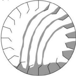
Figure 5.29 Overveiling – material pitches long.
