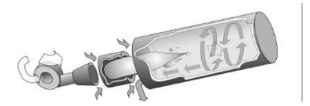
Figure 5.24 Older style burner with combustion chamber.
