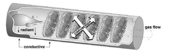
Figure 5.13 Three types of heat transfer in an aggregate dryer.
