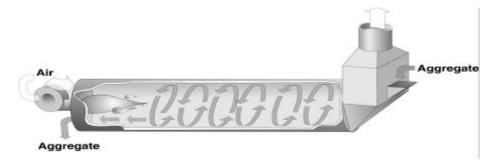
Figure 5.1 Typical counter-flow dryer.
