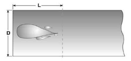
Figure 5.18 Combustion zone length equals diameter ratio.
