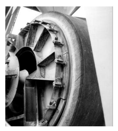
Figure 5.50 Mechanical type dryer seal.
