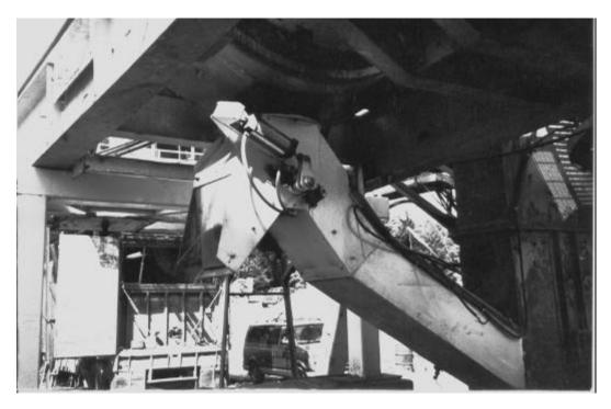
Figure 5.52 Gravity drop chute from dryer.
