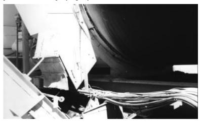
Figure 5.53 Sweep discharge on drum-mixer or dryer.
