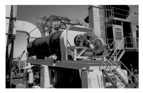
Figure 5.26 Older dryer with new combustion chamberless burner.
