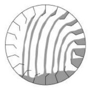
Figure 5.40 Proper rotational speed and balance of material across dryer-cross-section.
