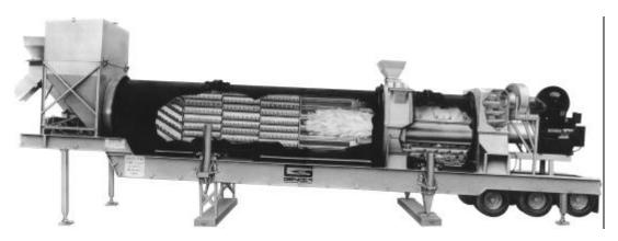
Figure 5.6 Counter-flow drum-mixer.
