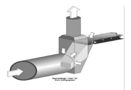
Figure 5.49 Belting type dryer seal.
