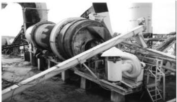
Figure 5.54 High-lift discharge on batch plant dryer.
