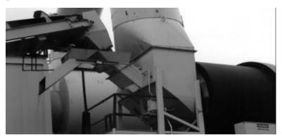
Figure 5.44 Fixed chute entry to dryer with vibrator on chute.
