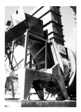
Figure 5.46 Rotating chute entry to dryer.
