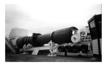
Figure 5.4 Parallel-flow drum-mixer.
