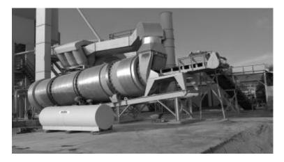
Figure 5.14 Counter-flow dryer with insulation.
