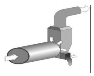
Figure 5.56 Tramp air being drawn in around parallel-flow dryer discharge area.
