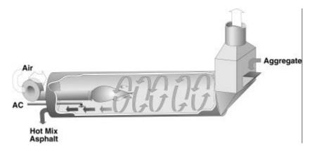
Figure 5.5 Typical counter-flow drum-mixer.
