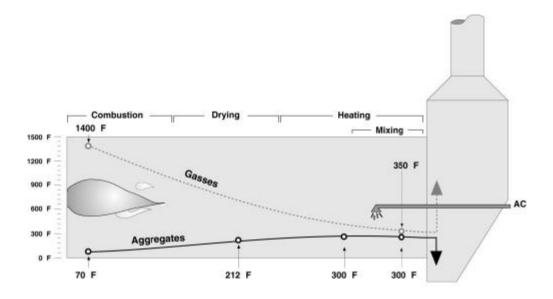
Figure 5.33 Temperature profile of parallel-flow drum mixer drying virgin aggregates.
