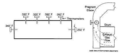
Figure 5.41 Measuring gas flow in the gas discharge ductwork provides an indication of veiling efficiency.
