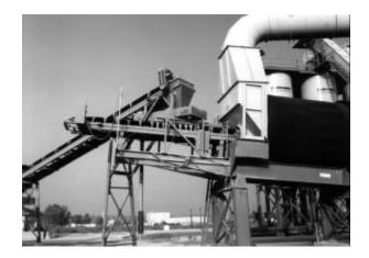
Figure 5.48 Slinger feed entry to counter-flow drum-mixer.
