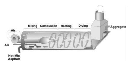
Figure 5.9 Counter-flow drum-mixer zones.
