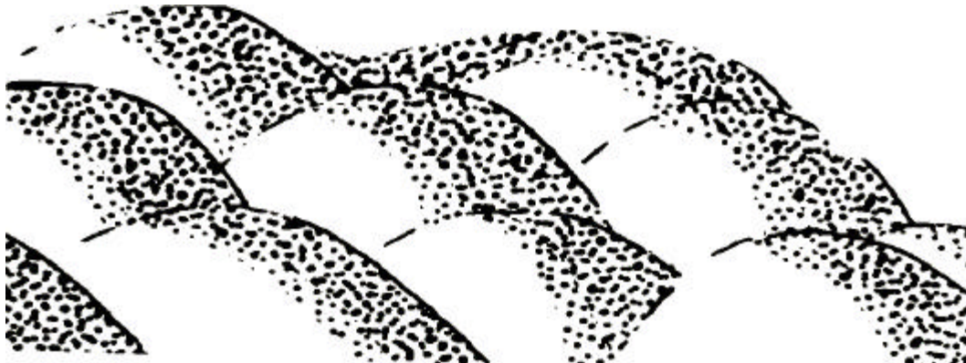
Figure 3.1 Horizontally stockpiled aggregate.
