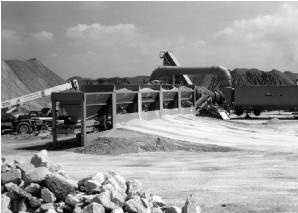
Figure 3.16 Material should not be heaped causing overflow.
