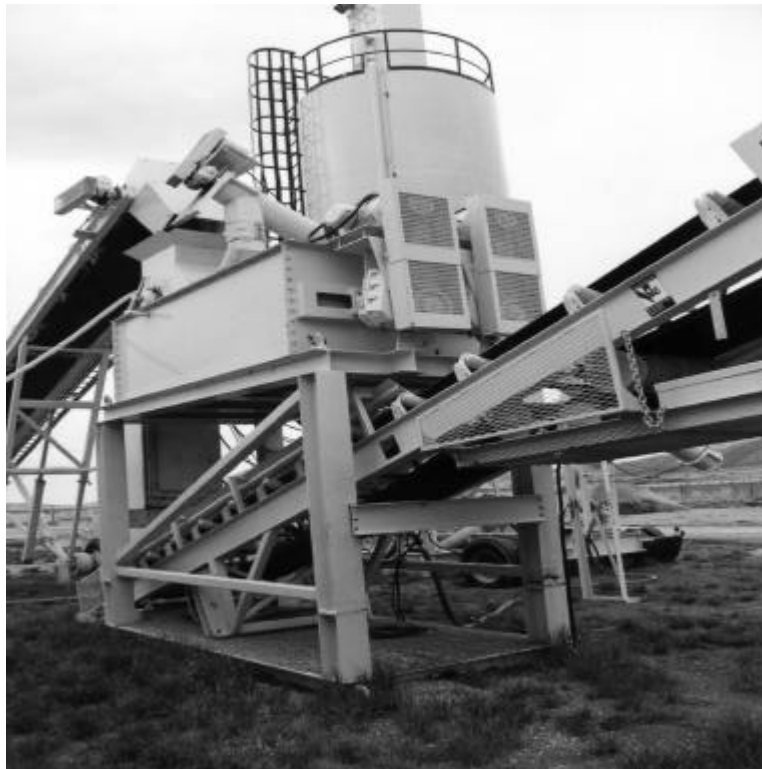
Figure 3.47 Continuous pugmill for mixing lime with aggregate prior to entry to dryer or drum-mixer.
