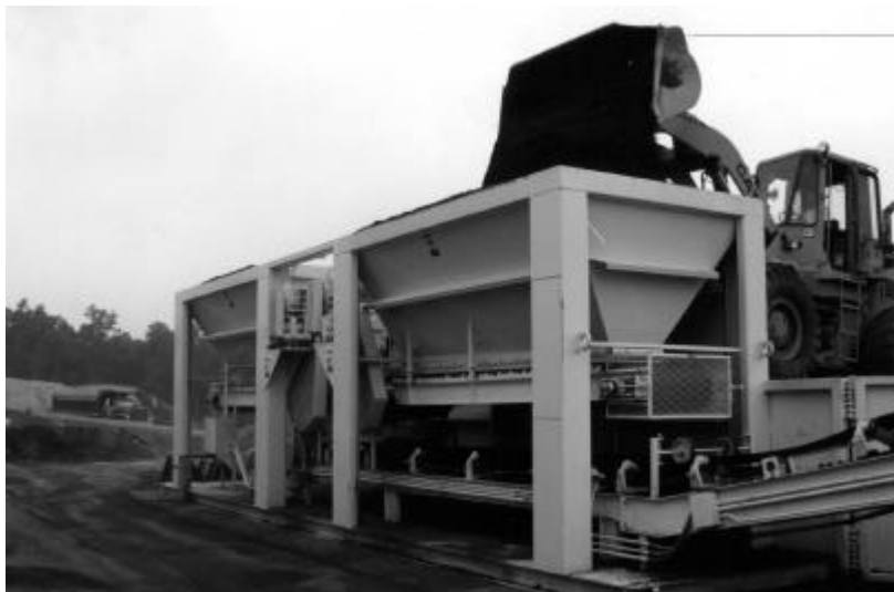
Figure 3.38 Twin RAP bin system with long RAP feeders.
