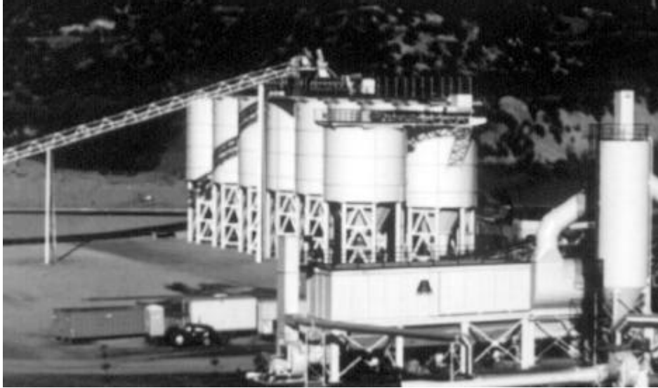
Figure 3.10 Covered and elevated bulk storage bins.
