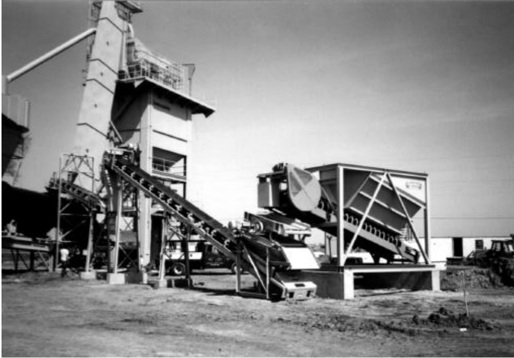
Figure 3.37 Incline RAP feeder.
