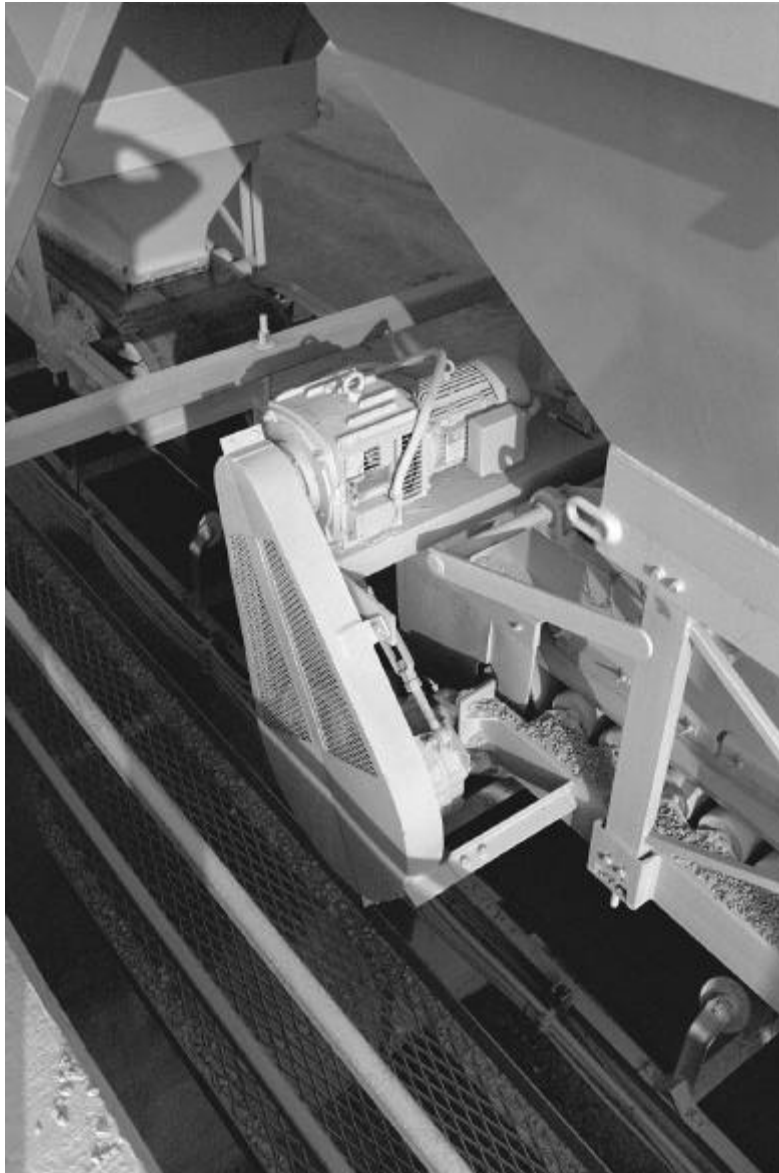
Figure 3.29 Feeder with TASC drive fitted to constant speed gearbox.
