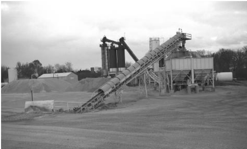
Figure 3.10 Covered and elevated bulk storage bins.
