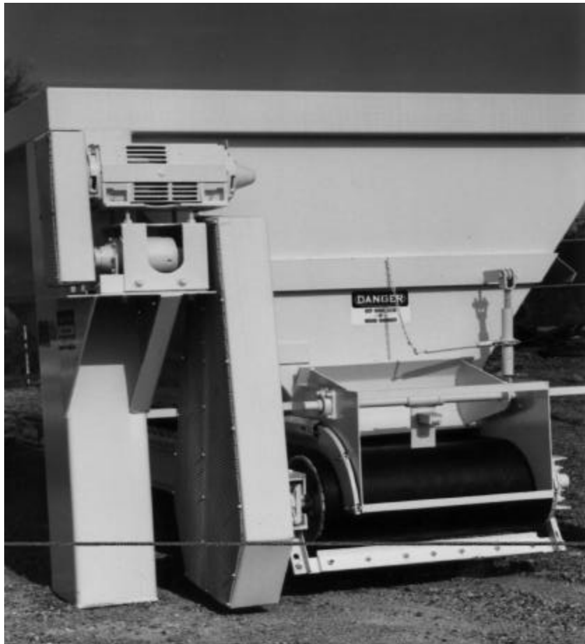
Figure 3.27 Feeder with DC motor and constant speed gearbox.
