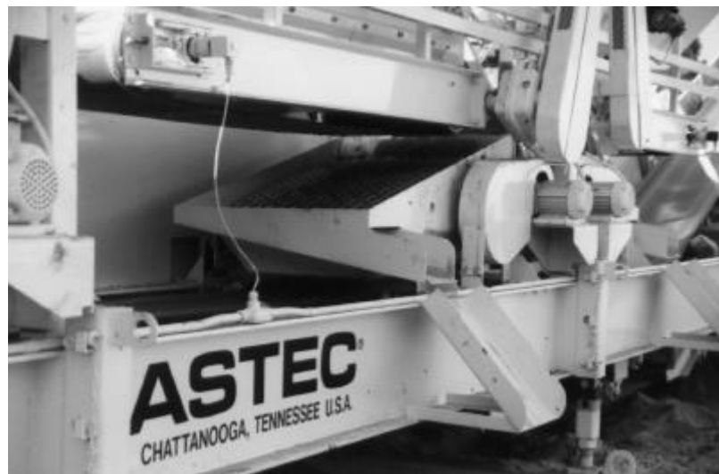
Figure 3.44 Cold feed system with scalping screens installed on each feed conveyor.
