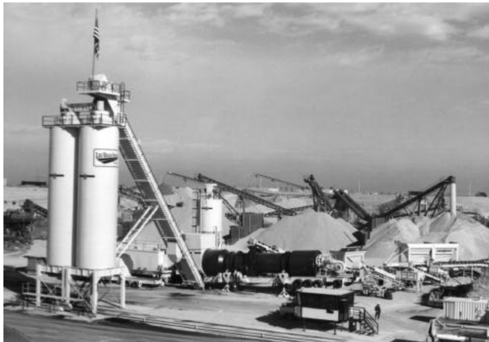
Figure 3.6 Radial stackers with truck dumping station.
