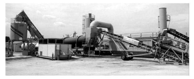
Figure 2.10 Modern counter-flow drum-mix facility.
