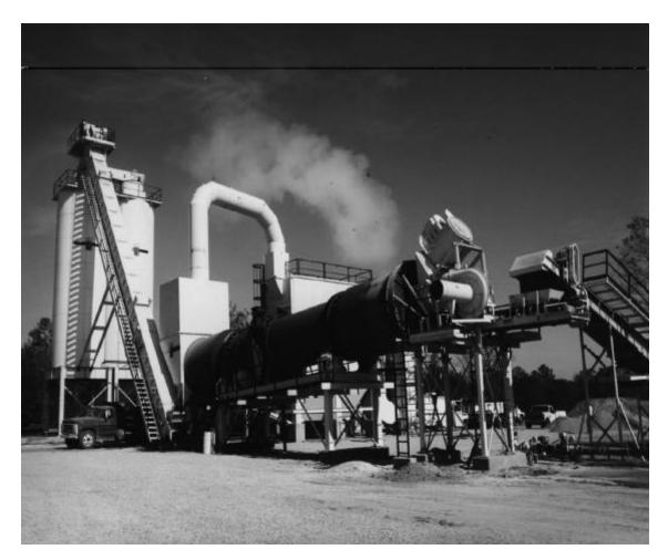
Figure 2.8 Modern parallel-flow drum-mix facility.
