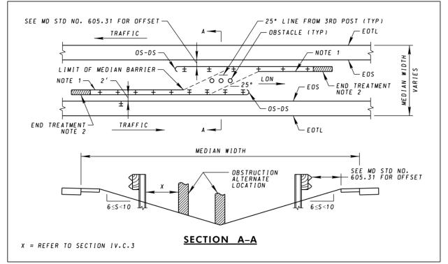
Note 1: If the back of the barrier is within the "Barrier Optional" or "Evaluate Need for Barrier" regions of Figure 6-1 of the RDG, a TBWB-MB is required
