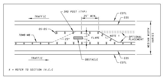
Note 1: For W-Beam traffic barrier, barrier should not be placed in areas that are not areas recommended in MD Std. No. 605.31 unless the slopes are modified as described in Section V of these Guidelines.
