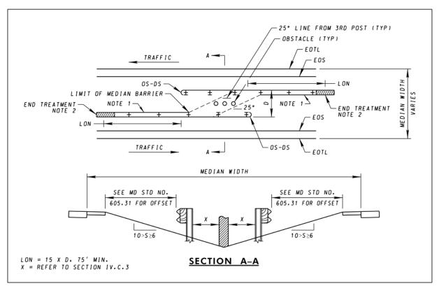
*Note 1: If the back of the barrier is within the "Barrier Option" or "Evaluate Need for Barrier" regions of Figure 6-1 of the RDG, a TBWB-MB is required*
