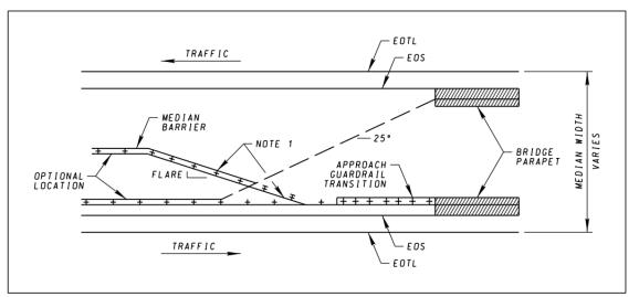
*Note 1: For W-Beam barrier, barrier should not be placed in areas that are not recommended in Std. MD-605.31 unless the slopes are modified as described in Section V of these Guidelines.*
