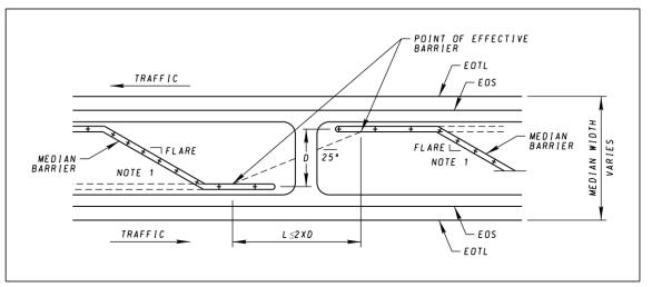
*Note 1: For W-Beam barrier, barrier should not be placed in areas that are not recommend in Std. MD-605.31 unless the slopes are modified as described in Section V of these Guidelines.*
