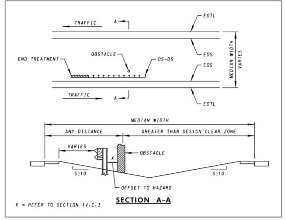
Note 1: If the end treatment is 35 feet or less from the opposing traffic, use a two-sided end treatment if the barrier is a TBWB-MB. Do not use a two-sided end treatment to end single face W-Beam in the median.
