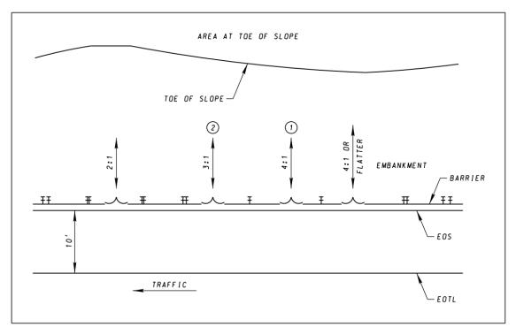
Figure 7: Example: Critical Embankment
