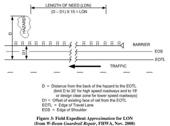
If there is a significant difference between the LON determined using the above procedure and either the existing or proposed installation location, the site should be reviewed to ensure appropriate application of LON.
