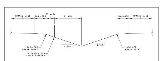
Figure 5: High-Tension Cable Barrier Placement on Slopes of 6:1 to 4:1
