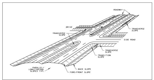
Figure 1: Roadside Slopes (Adapted from Figure 3-1 of the RDG) Source: AASHTO Roadside Design Guide, 4<sup>th</sup> Edition
