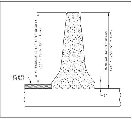
Figure 17: Pavement Resurfacing Considerations for Concrete Barrier
