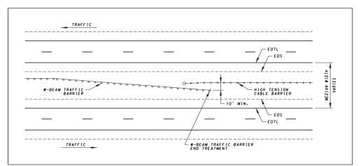
Figure 6: High-Tension Cable Barrier/W-Beam Traffic Barrier Transition Layout
