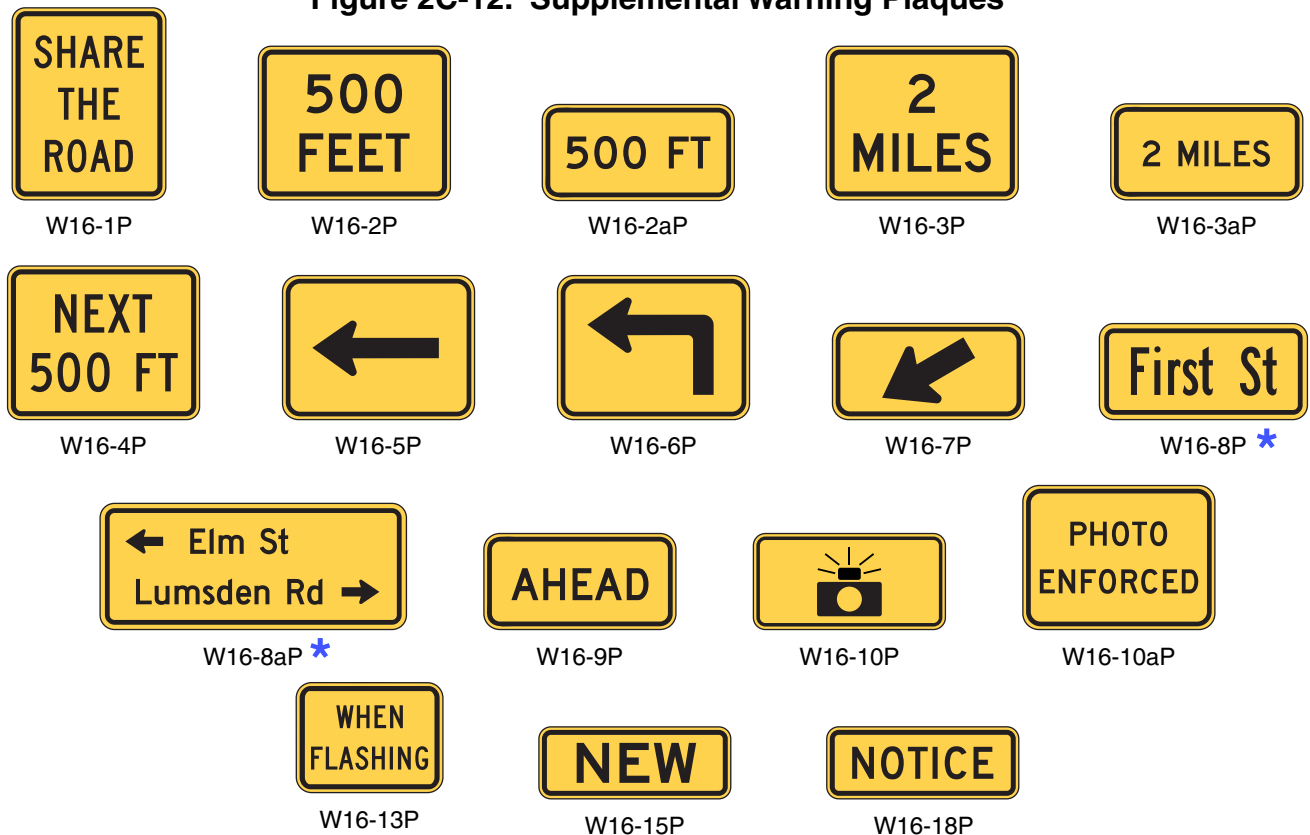
Figure 2C-12. Supplemental Warning Plaques
