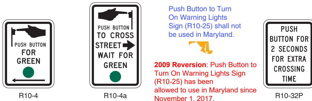
Figure 2B-26. Pedestrian Signs and Plaques (Sheet 2 of 2)
