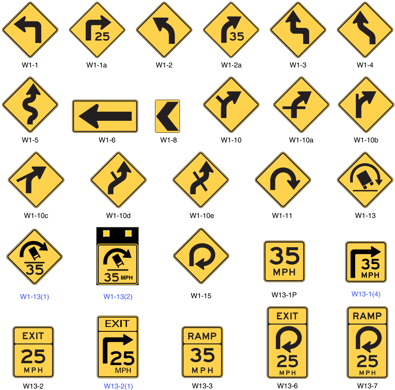
Figure 2C-1. Horizontal Alignment Signs and Plaques
