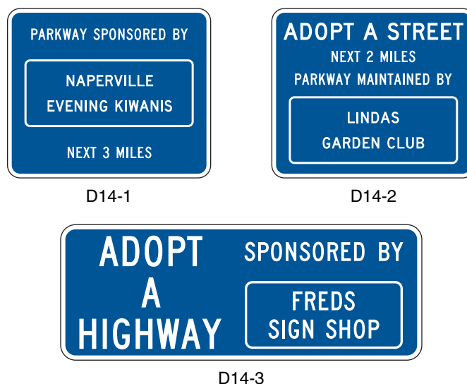
Figure 2H-5. Examples of Acknowledgment Sign Designs
