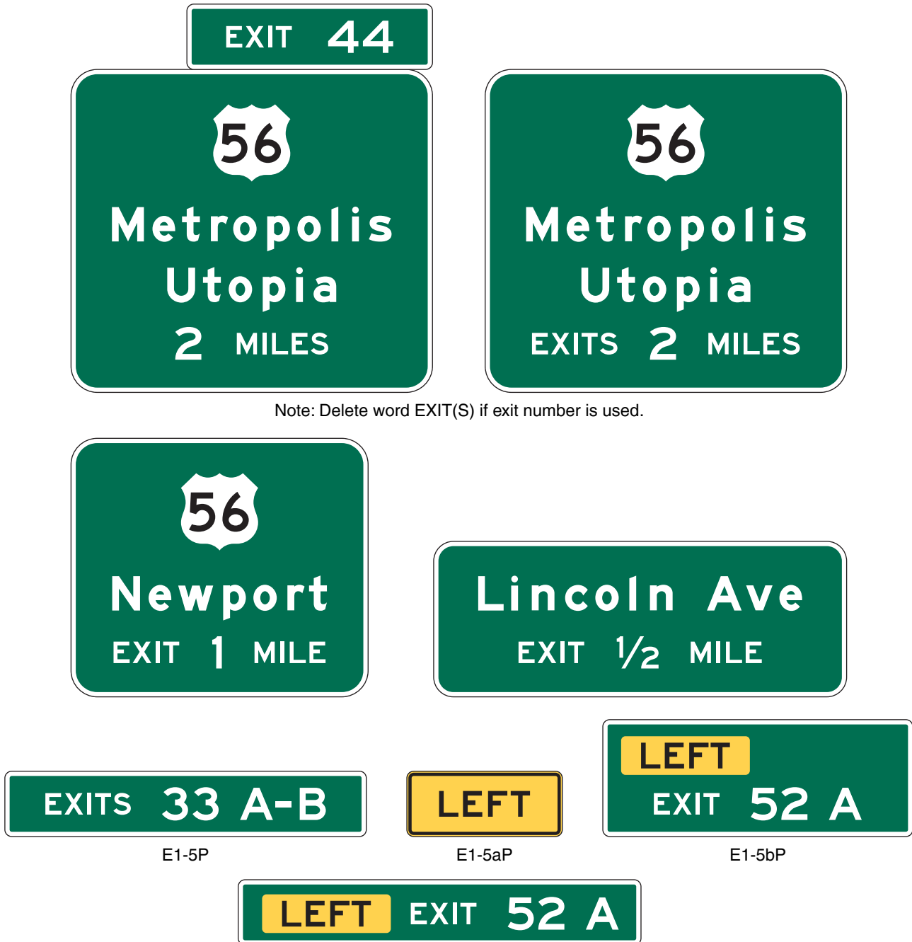
Figure 2E-22. Examples of Interchange Advance Guide Signs, Exit Number Plaques, and LEFT Plaque
