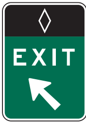
Figure 2G-14. Exit Gore Sign for a Direct Exit from a Preferential Lane
