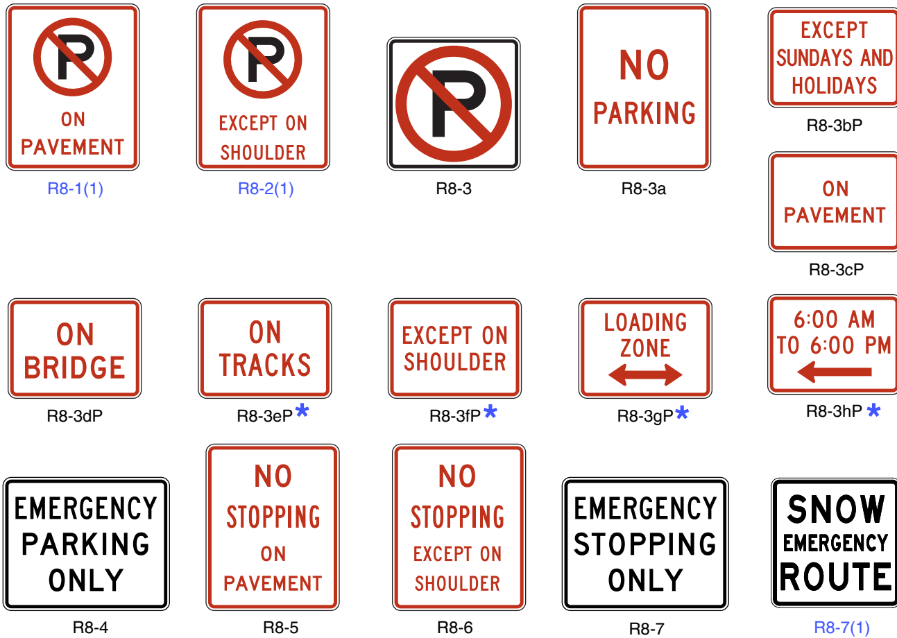
Figure 2B-25. Parking and Stopping Signs and Plaques (R8 Series)
