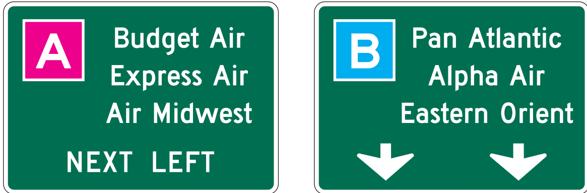
Figure 2D-1. Examples of Color-Coded Destination Guide Signs
