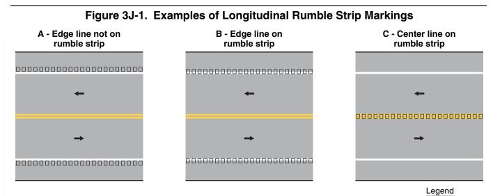
Note: Edge line may be located alongside the rumble strip (Option A) or on the rumble strip (Option B). Center line markings may also be located on a center line rumble strip (Option C).
