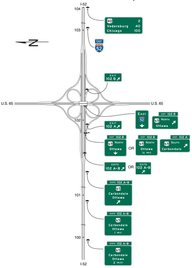
Note: See Figure 2D-15 for examples of multi-lane crossroad signing for a cloverleaf interchange
