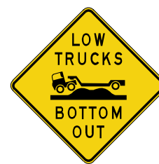
Figure 2C-13a. Low Trucks Bottom Out Sign
