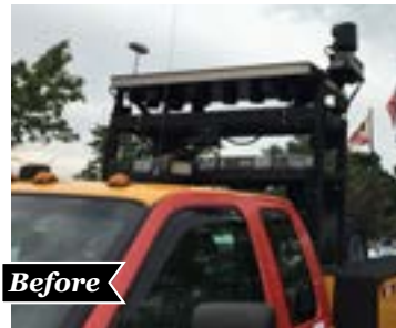
Dave Rineholt discovered that moving the bracket to the inside provides a more stable mount that better protects the camera equipment.
