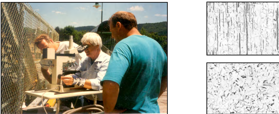
Figure 1. Non-destructive metallographic examination (left) can be used to identify the microstructure of wrought iron (top right) versus steel (bottom right). Note the distinctive elongated slag fibres in the wrought iron.
