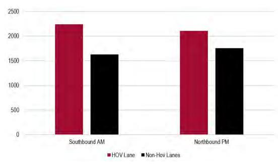
Figure II-11 I-270 AVERAGE PERSON THROUGHPUT PER LANE PER HOUR
