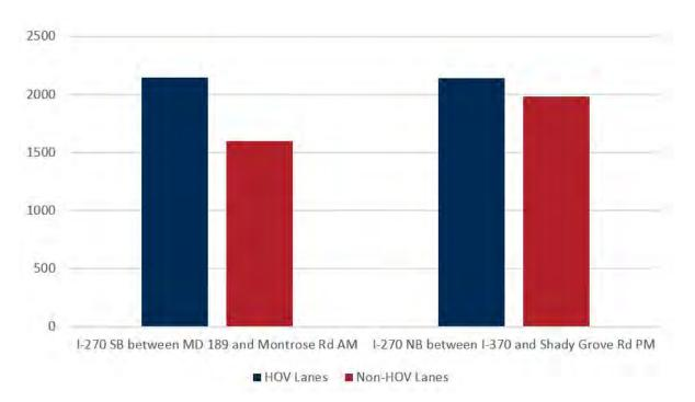
FIGURE II-11 I-270 PERSON THROUGHPUT PER LANE PER HOUR
