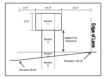
Figure EE.1 - Ground Mounted Support Lengths July 2017
