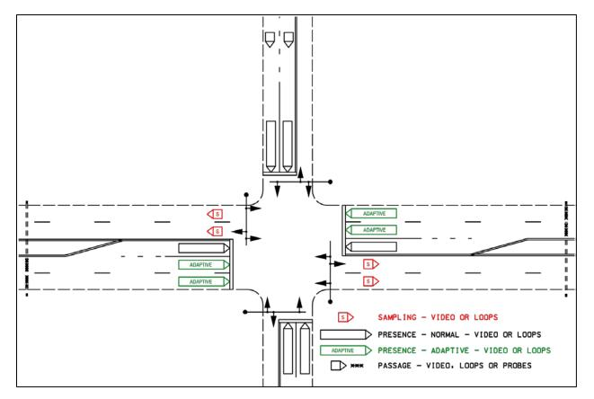
Figure SG. 26 - Detection Zone Types
