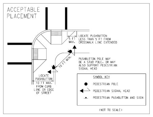
Figure SG. 31 - Acceptable Placement of APS
