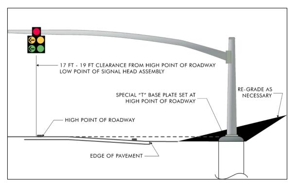
Figure SG. 6 - Special "T" Dimension Mast Arm Installation
