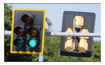
Figure SG. 14 - Signal Backplates
