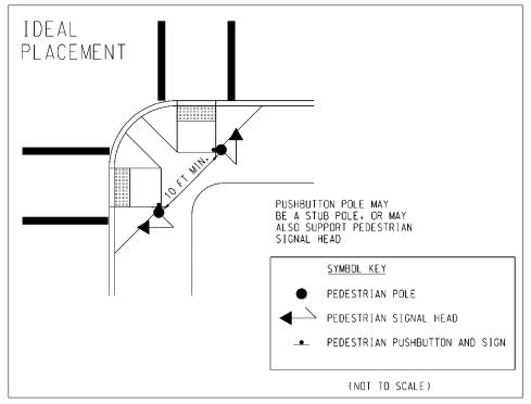
Figure SG. 32 - Ideal Placement of APS
