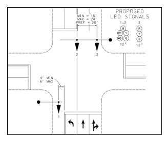
Figure SG. 16 - Signal Head Horizontal Placement – Typical Signal Head Placements for Exclusive/Permissive Left Turn
