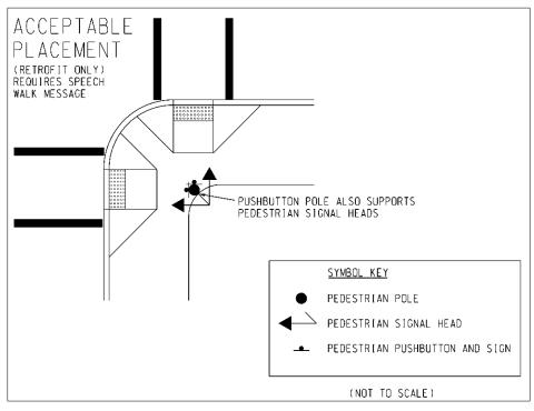
Figure SG. 33 - Retrofit Placement of APS
