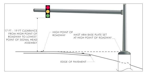
Figure SG. 5- Mast Arm Installation
