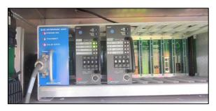
Figure SG. 40 - 4-Channel Vehicle Detector Amplifiers
