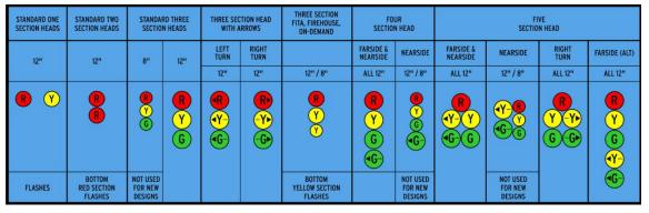
Figure SG. 13 - Signal Head Arrangements
