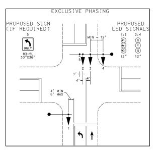
Figure SG. 17 - Preferred near and far side three section heads with arrows and two threesection standard heads
