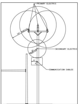
Figure SG. 9 - Overhead Utility Locations and Clearances
