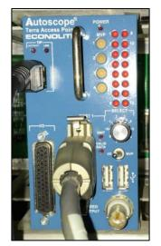
Figure SG. 20 - Video Interface Card (Close Up)
