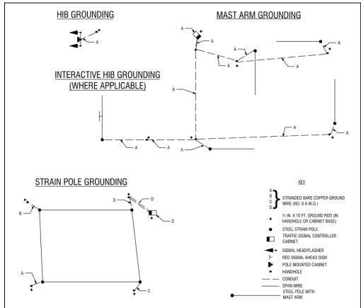
Figure SG. 35 - Grounding Diagram
