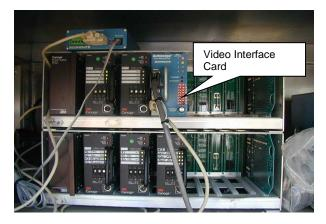
Figure SG. 21 - Rack Mounted Video Interface Card
