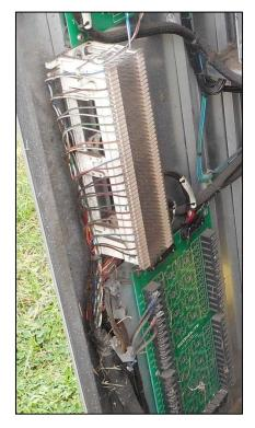
Figure SG. 41 - 12-Pair Interconnect Cables
