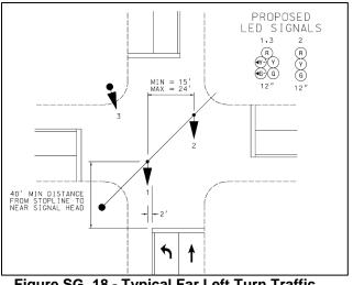
Figure SG. 18 - Typical Far Left Turn Traffic Signal Head Location\*
