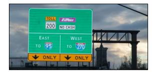
Figure SN.10 - Negative Contrast "ONLY" Panels
