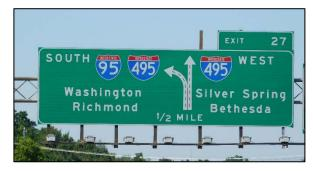
Figure SN.11 - Typical Diagrammatic Sign
