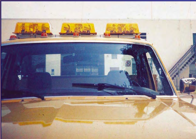
Rotating/flashing Yellow Warning Lights
