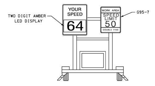
Figure 1. Preferred speed display configuration.
