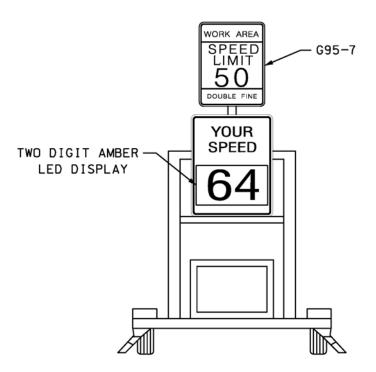
Figure 2. Speed display configuration to be used on roadways with lateral restrictions.
