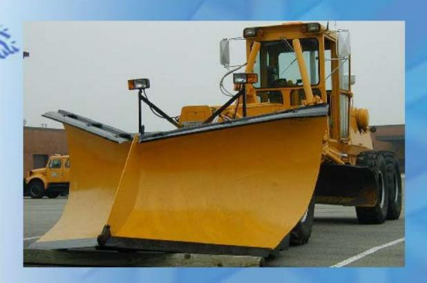
V-Plows are mounted to a Grader or Oshkosh.
