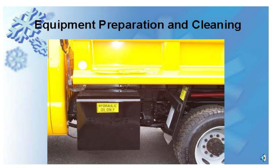
Check all fluid systems for leaks to reduce the risk of discharge of petroleum-based products on roadways and macadam (paved) lots.
