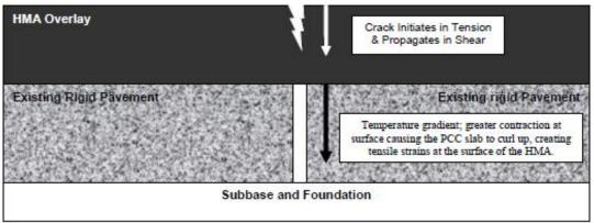
Figure 11: Thermally-induced Cracking; Curling of PCC Slab
