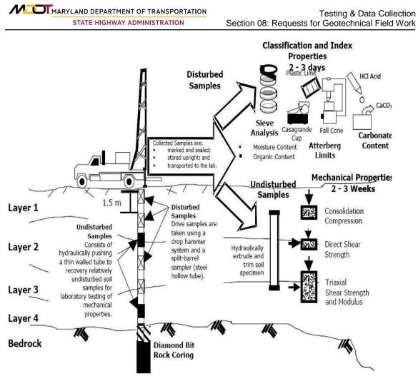
Figure 8: Traditional Drilling, Sampling, and Laboratory Testing of Collected Samples (Courtesy: FHWA-IF-02-034, Geotechnical Engineering Circular No. 5, Evaluation of Soil and Rock Properties)
