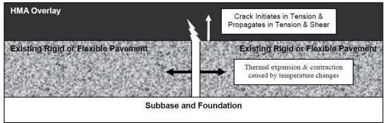
Figure 9: Thermally-Induced Reflective Cracking; Horizontal Movements
