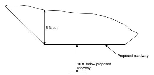
Figure 7: Boring Depth in Cut Areas
