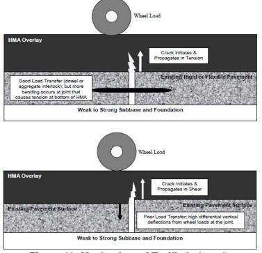
Figure 10: Mechanism of Traffic-induced Reflective Cracks of HMA Overlays
