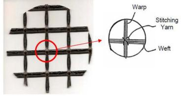
Figure 12: Structure of a Fiber-glass Grid
