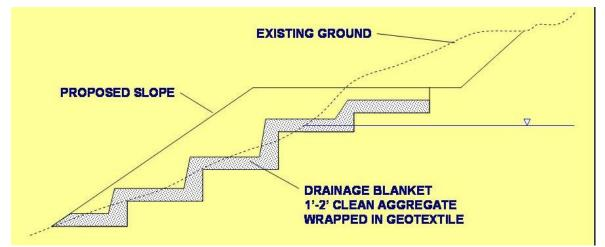
Drainage Blanket Example – Wet Soil or Wet Cut Areas
