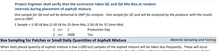
When daily placed quantity of asphalt mixture is low (<200 ton) samples of the asphalt mixture will be taken less frequently. These will occur at random intervals behind the paver and be analyzed at the respective laboratories. Results will be utilized in determining a mixture pay factor and statistical analysis, the producer's data is only included if the sample was taken behind the paver. If multiple mix formulations are utilized the frequencies indicated are for each mixture that is placed.
