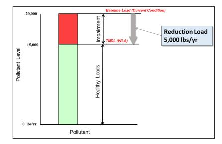
Figure 3-6: Example Wasteload Allocation and Reduction Requirement
