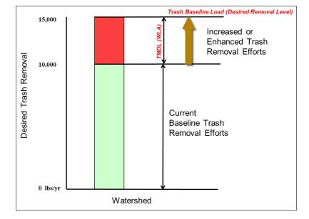
Figure 3-10: Trash TMDL Baseline and WLAs
