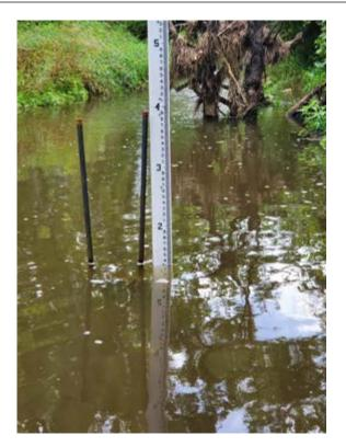
*Figure 4. FY22 relocated downstream station (Site ID 01636846) on Little Catoctin Creek near Rosemont, MD. The photo shows the HOBO logger and stream gage.*
