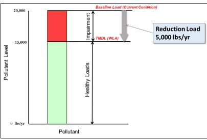
Figure 3: Example Wasteload Allocation and Reduction Requirement
