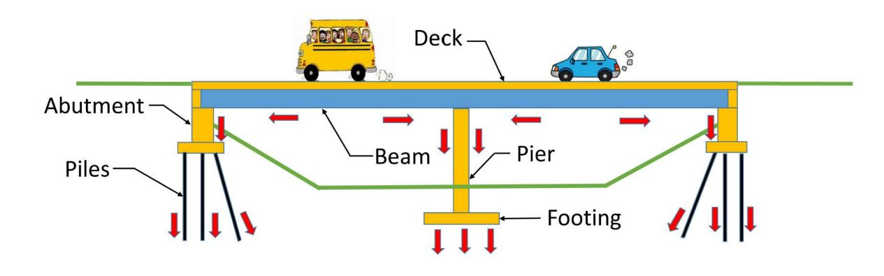
This diagram shows the names for different parts of a bridge. The arrows show how forces are directed between the bridge parts so that the bridge stays standing and supports its loads.
