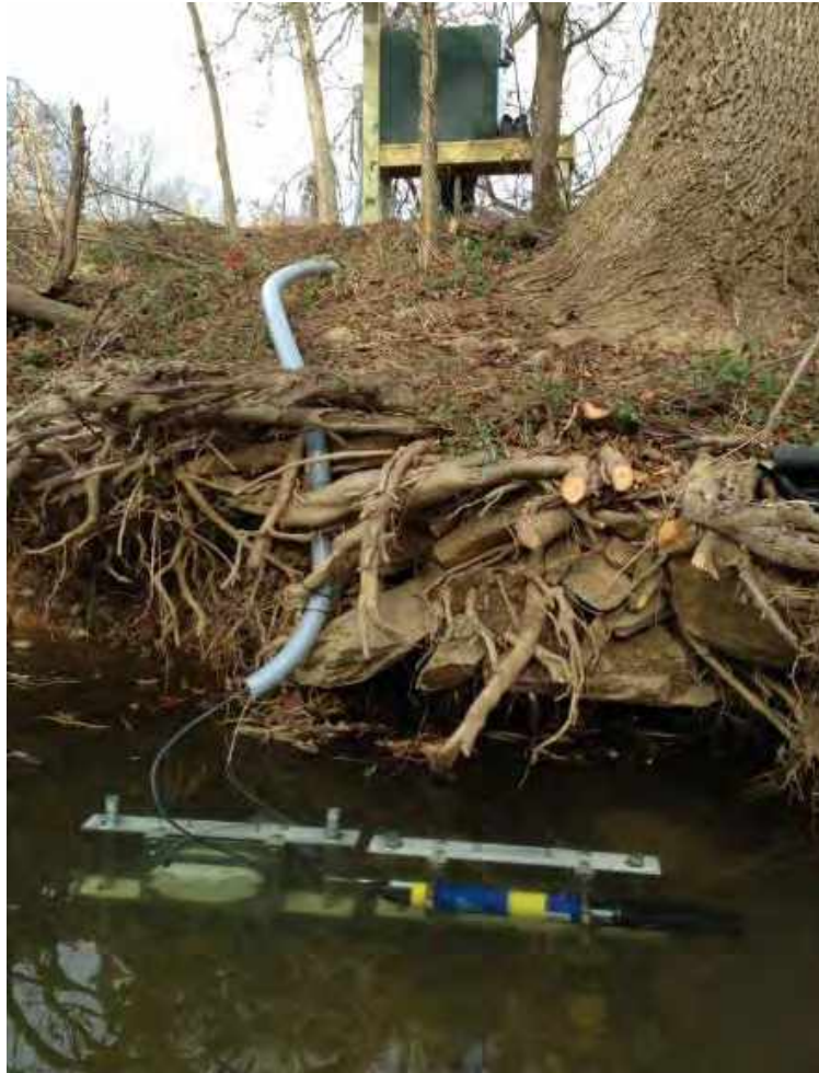
Figure 5. U.S. Geological Survey the downstream station (Site ID 01636846) on Little Catoctin Creek near Rosemont, MD. The photo shows the temporary gage station and the discharge and water-quality sonde installed in the river.
