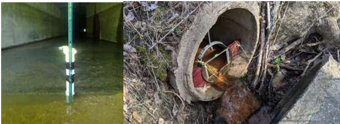
Figure 3. Depth logger mounted at box culvert bottom upstream of I-70 (left; Flow Station 1) and at the outfall of the proposed ESDs with weir (right; Flow Station 2)
