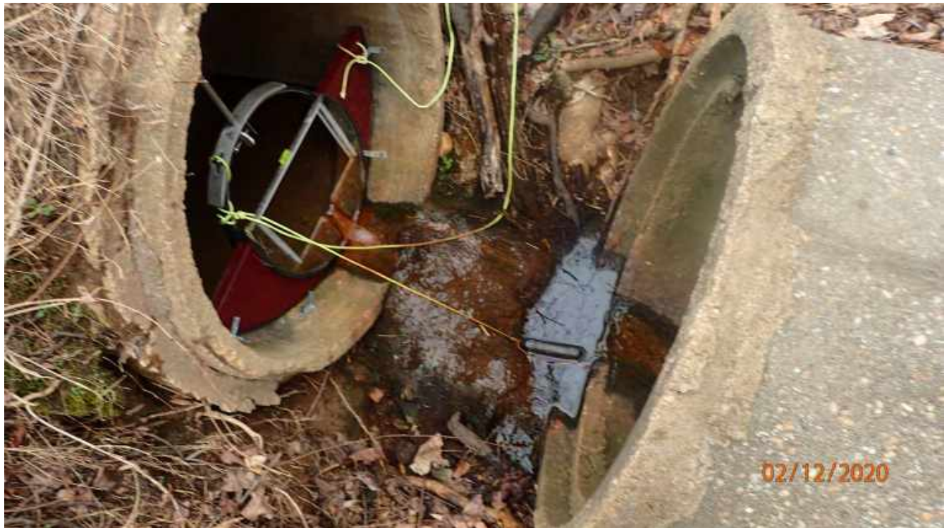
Photograph 130. 2/12/2020 Year 3 Monthly Download and Maintenance, Flow Station 2, logger replaced
