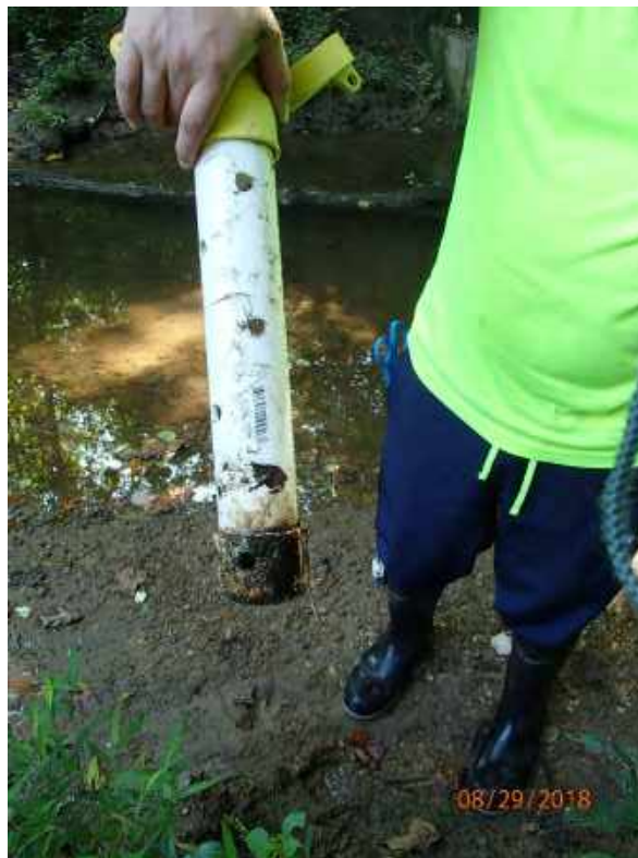
Photograph 18. 8/29/2018: Sediment being cleaned out of Flow Station 1 housing
