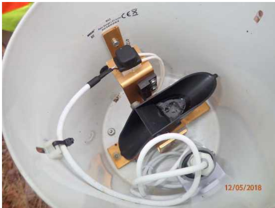
Photograph 62. 12/05/2018: Rain gauge tipper with collected ice, monthly download before maintenance
