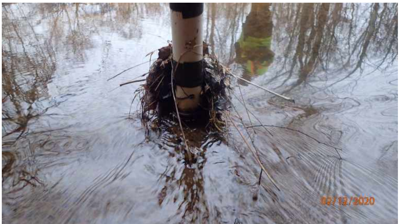
Photograph 134. 2/12/2020 Year 3 Monthly Download and Maintenance, Flow Station 1 with debris before maintenance
