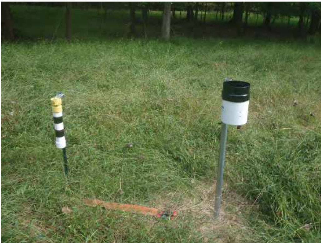
Photograph 52. 10/08/2018: Barometer and rain gauge, monthly download. Before maintenance
