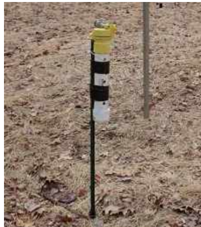
Figure 4. Barometric pressure logger set-up
