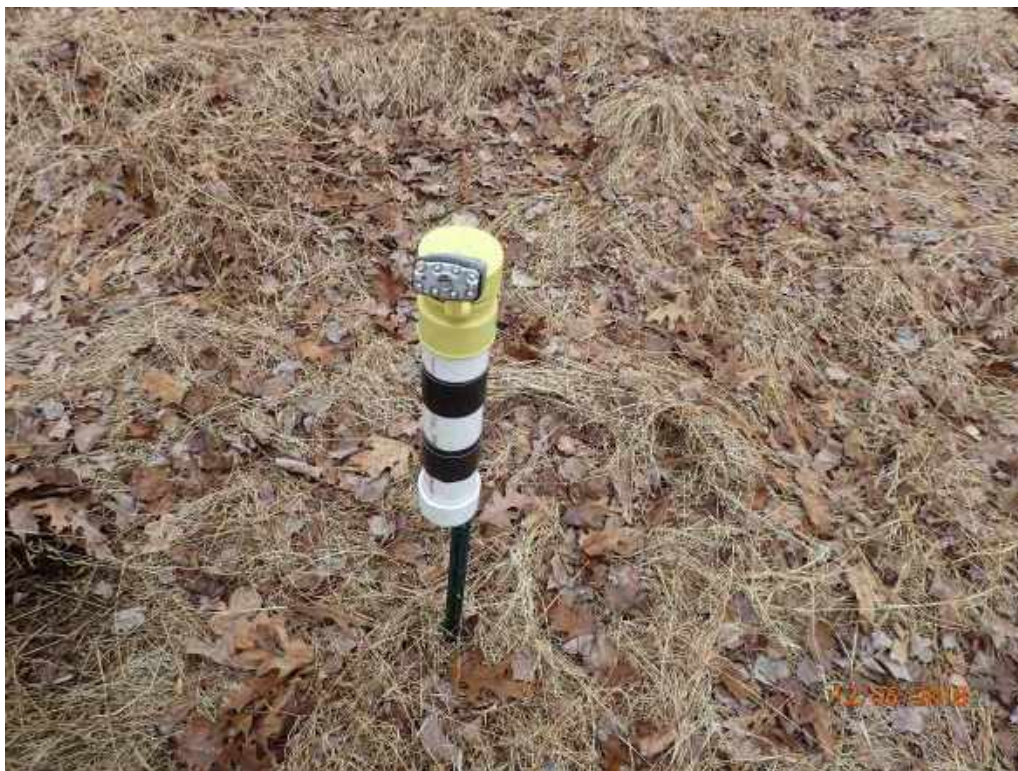
Photograph 60. 12/05/2018: Barometer, monthly download before maintenance
