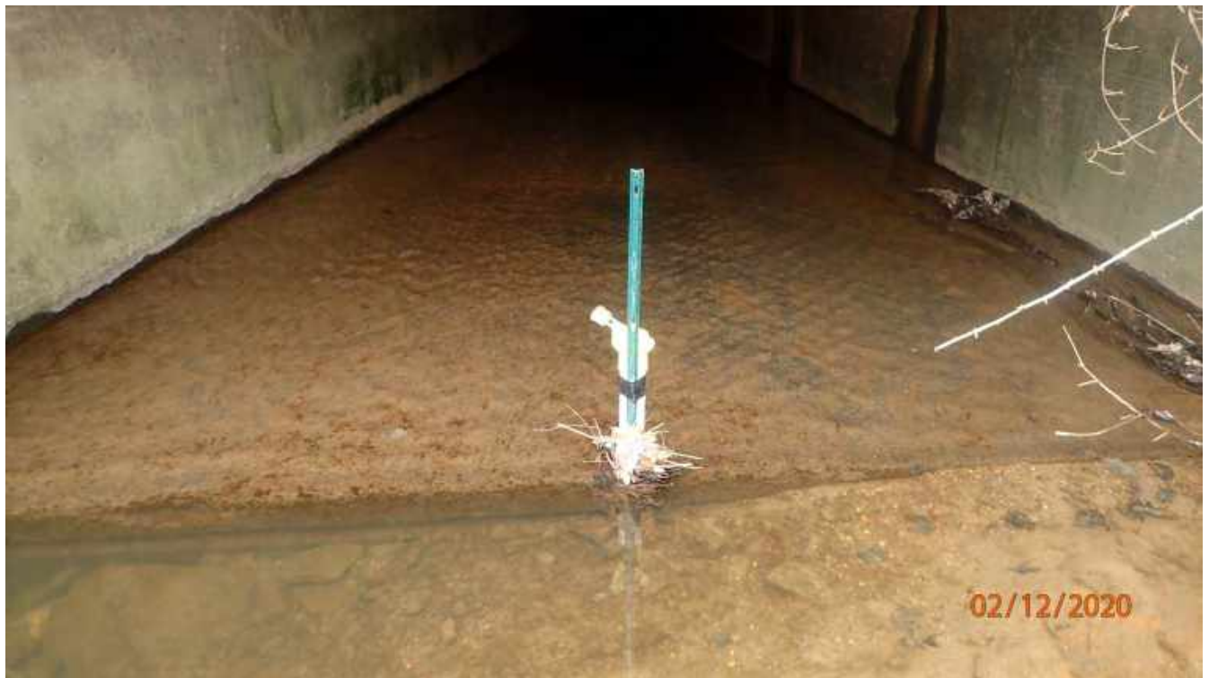
Photograph 134. 2/12/2020 Year 3 Monthly Download and Maintenance, Flow Station 1 with debris before maintenance
