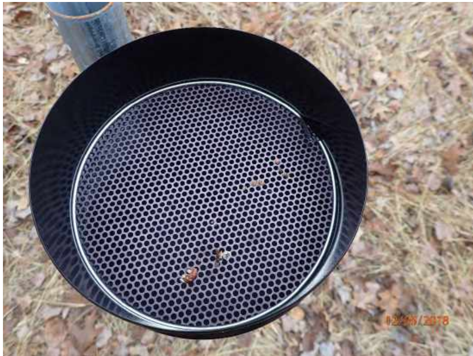
Photograph 62. 12/05/2018: Rain gauge tipper with collected ice, monthly download before maintenance
