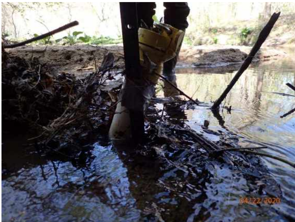
Photograph 148. 4/22/2020: Year 3 Monthly Download and Maintenance, Flow Station 1, dislodged and out of position under weight of debris
