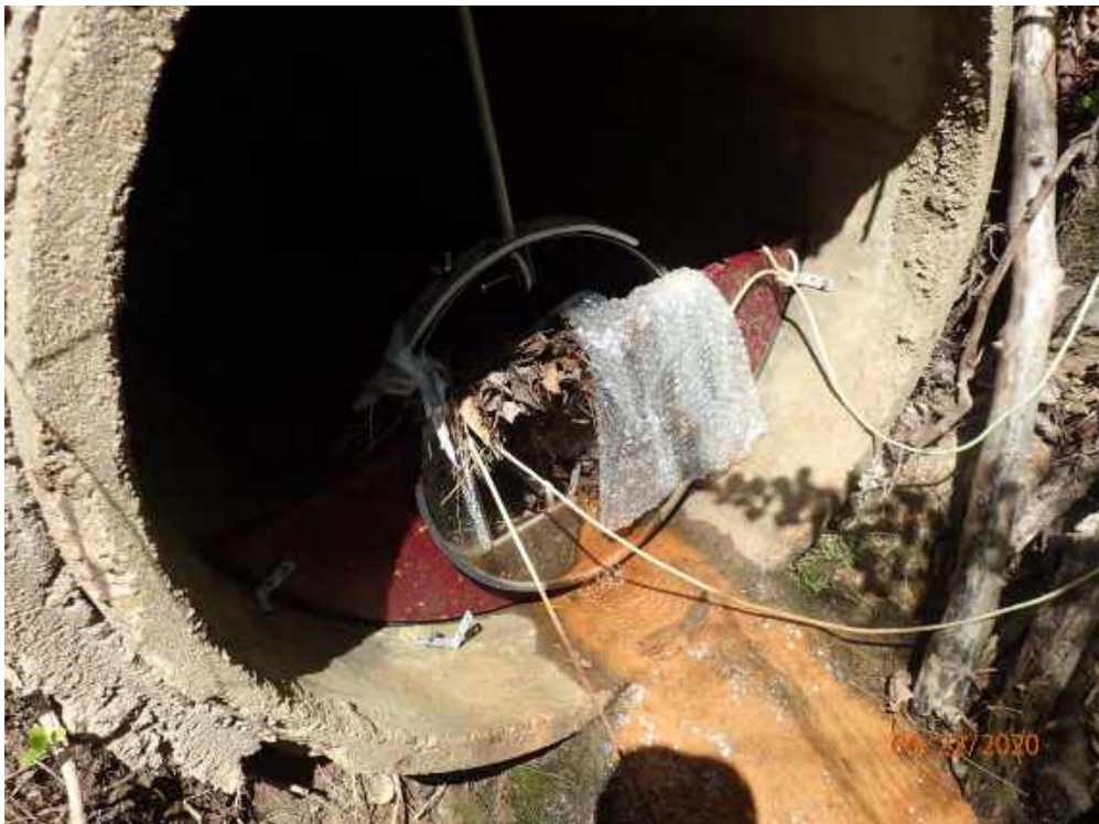
Photograph 140. 4/22/2020: Year 3 Monthly Download and Maintenance, Flow Station 2 with debris build-up
