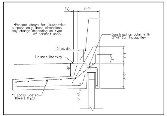
Figure 2-8: Barrier Doweled into Moment Slab
