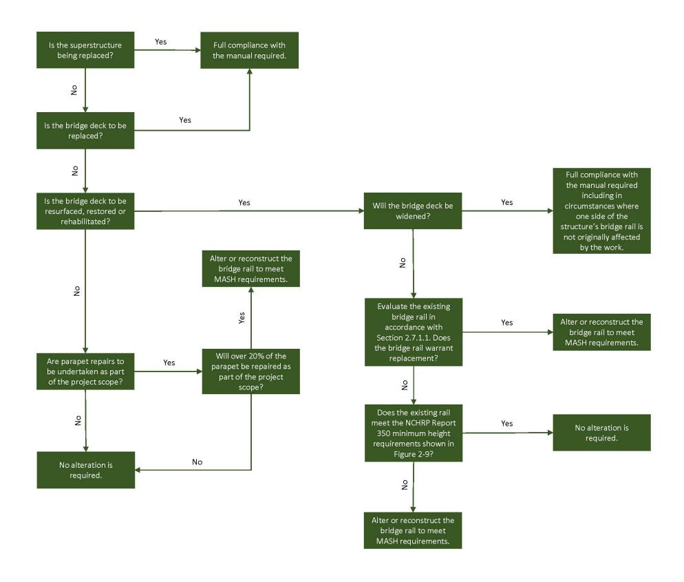
Figure 2-10: Treatment of Existing Bridge Rail
