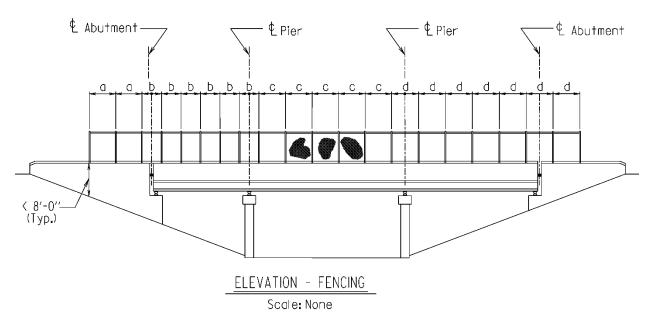
Figure 2-6: Fence Spacing on Bridges
