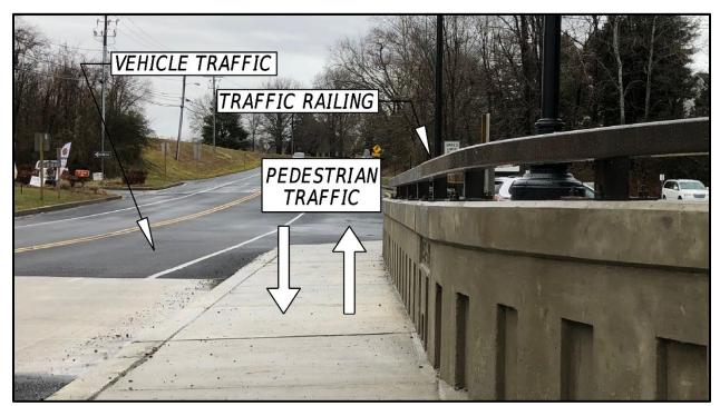
Figure 2-2: Low-Speed Roadway with Pedestrian Facility
