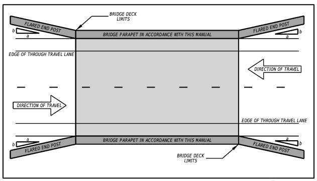
Figure 2-4: Tapered End Posts at Locations where Aesthetics is a concern and there is no Adjacent Traffic barrier
