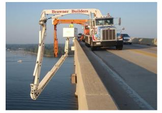
Figure 8. Under-Bridge Inspection Vehicle
