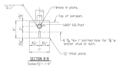
\* For Special Parapets outside face of parapet to be formed with a 8" wide recess, perpendicular to top of parapet, to accept anti-climb shield base plate. Recess to be 5" long measured from top of parapet.
