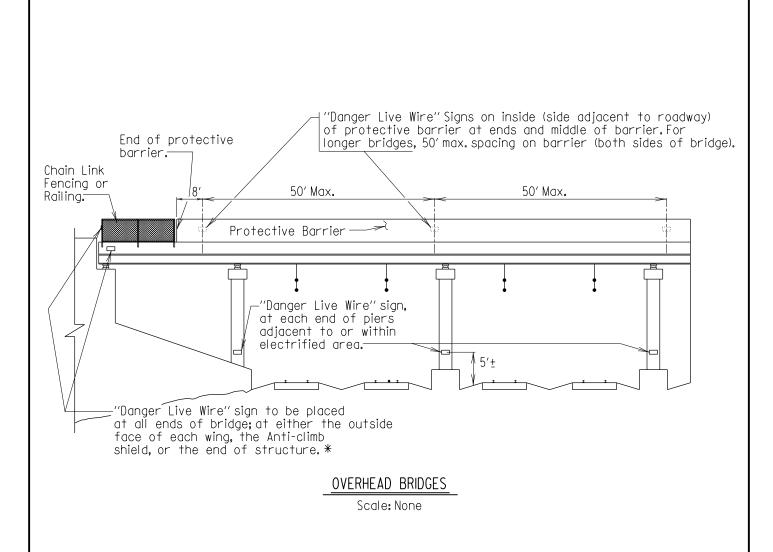
\* Where structure is of multispan configuration and end of bridge is a considerable distance from electrified areas (over 200' from electrified span) additional signs shall be placed in spans just adjacent to electrified span(s).
