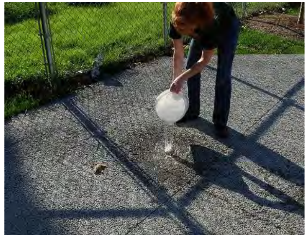
Permeable pavement examples with interlocking pavers and porous bituminous asphalt
