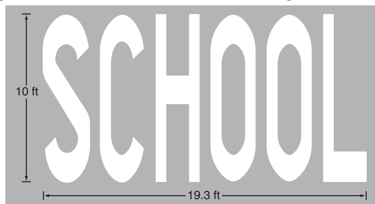
Figure 7C-1. Two-Lane Pavement Marking of “SCHOOL”
