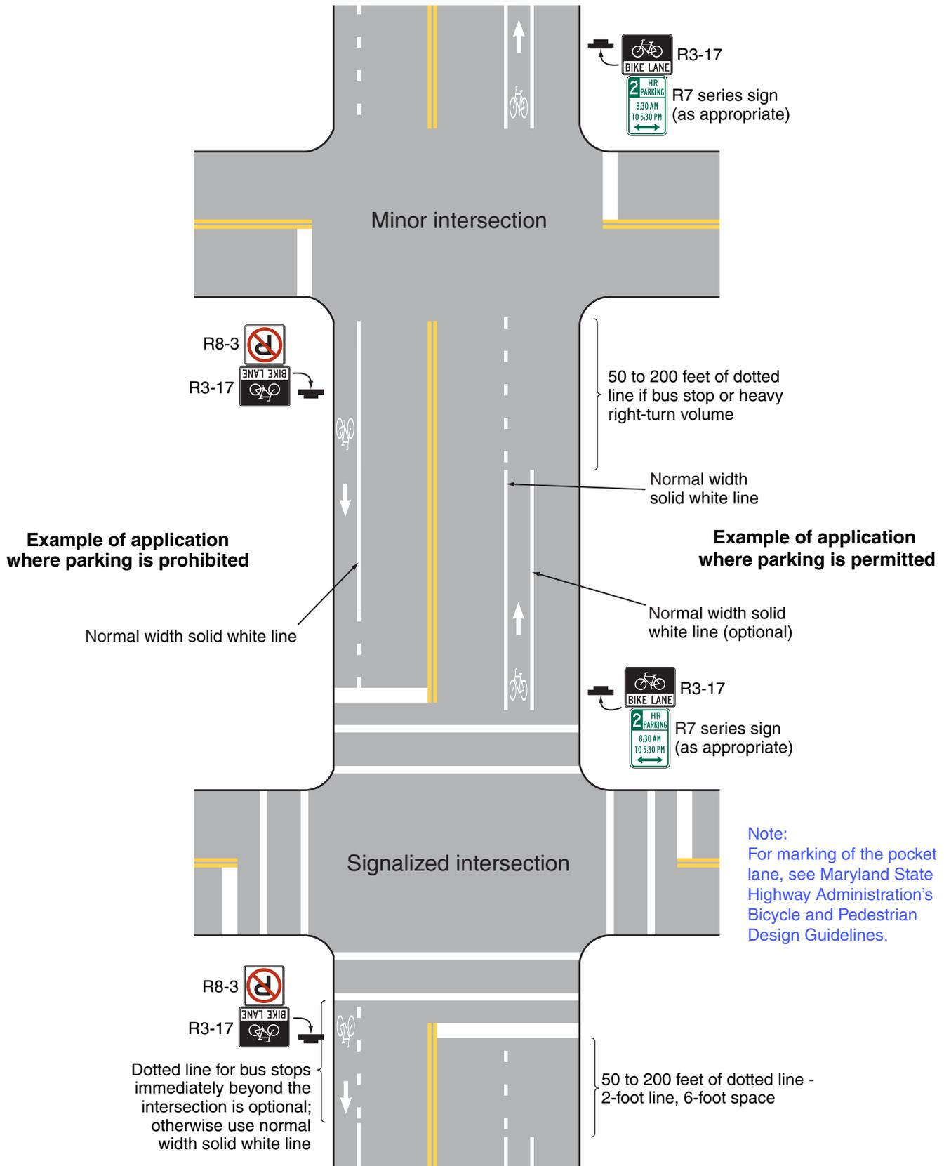
**Figure 9C-6a. Example of Typical Shoulder Bicycle Lane Changes to Right Turn Lane Without Pocket Lane**
