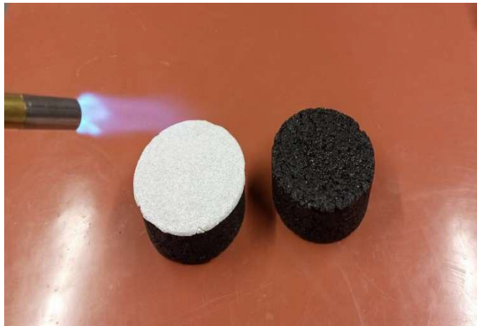
Figure 3.2: Application of Preformed Thermoplastic on Asphalt Surfaces
