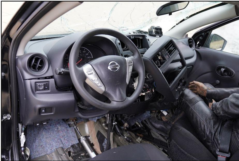
**Figure 6.10. Interior of Test Vehicle on Impact Side after Test 614271-12-2.**
