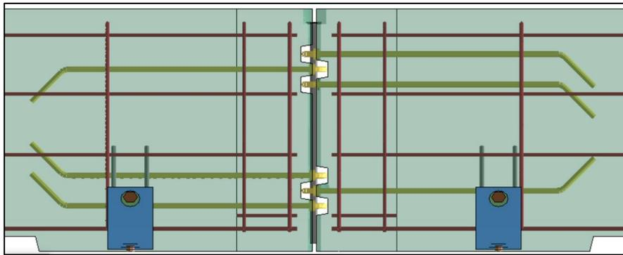
**Figure 2.14. Reinforcement Details of Modified Barrier Model.**
