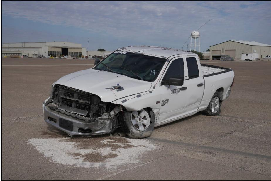
**Figure 7.7. Impact Side of Test Vehicle after Test 614271-12-1.**
