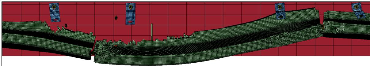
**Figure 2.10. Concrete and Anchorage Damage after *MASH* Test 3-11 Impact (Top View).**
