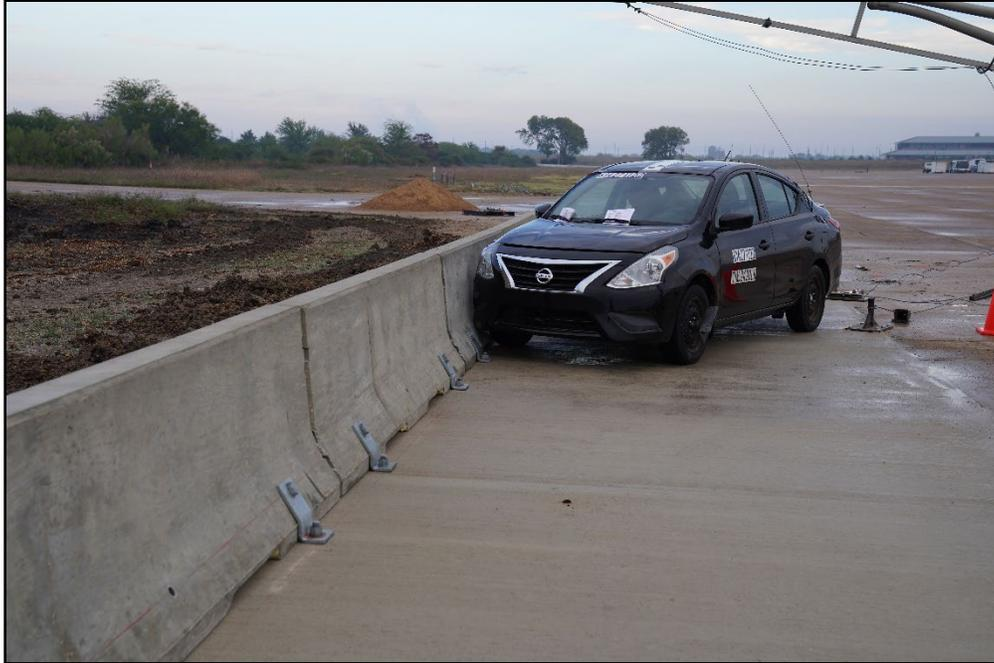
**Figure 6.1. Maryland F-Type Temporary Barrier and Test Vehicle Geometries for Test 614271-12-2.**
