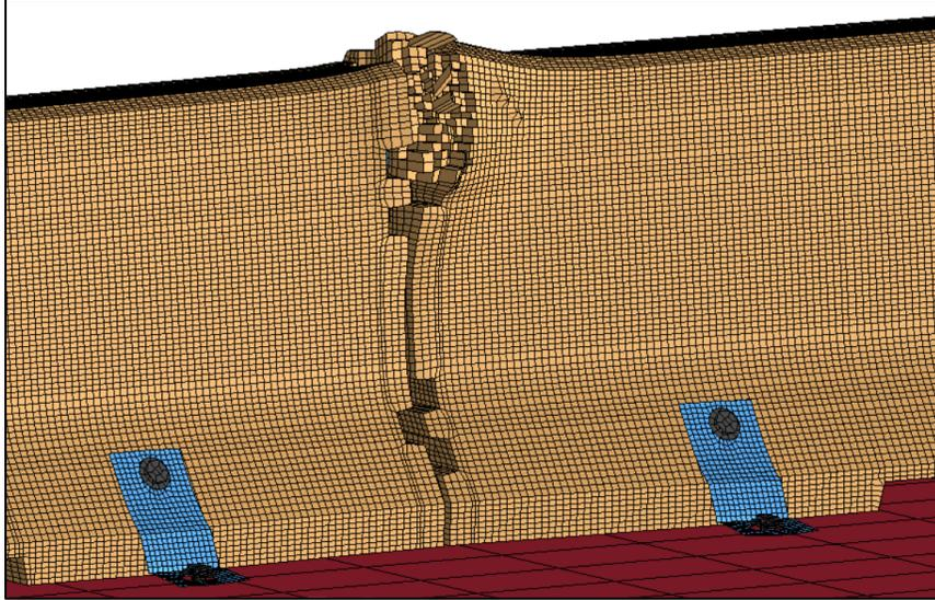
**Figure 2.18. Isometric View of Impacted Area after *MASH* Test 3-11.**
