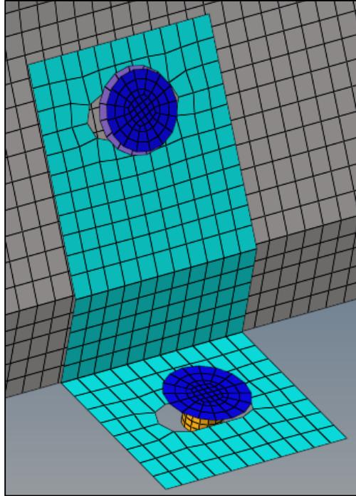
**Figure 2.7. FE Model of Hold-Down Anchor Plate.**
