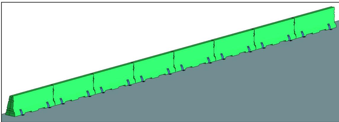
**Figure 2.15. Modified Barrier System with Eight Segments.**
