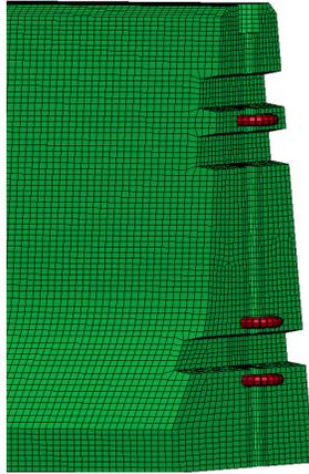
**Figure 2.13. Isometric View of Modified Barrier Segment FE Model.**
