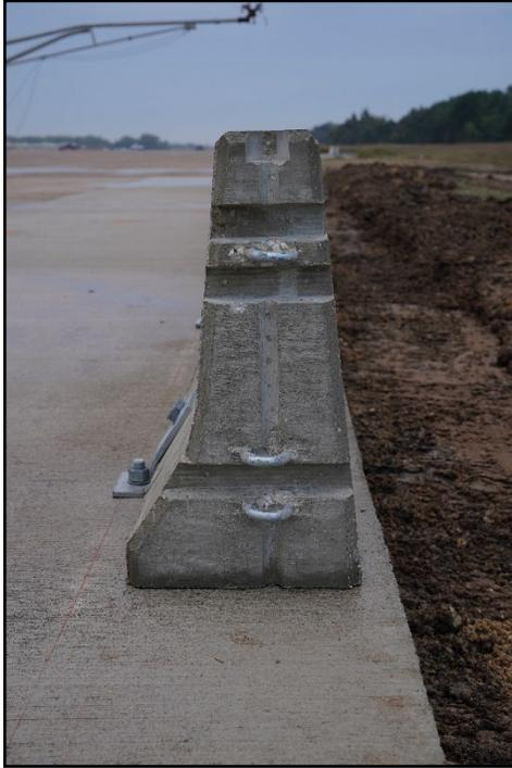
**Figure 3.4. Maryland F-Type Temporary Barrier prior to Testing—Lateral View of the Installation.**
