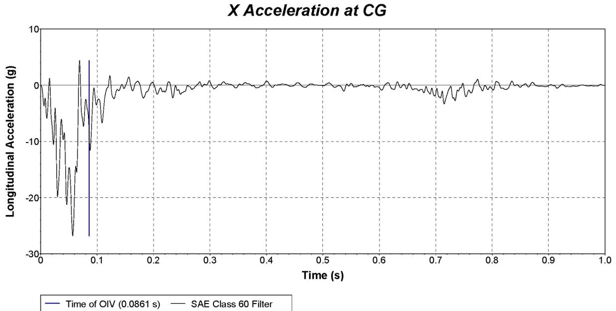
**Figure C.8. Vehicle Longitudinal Accelerometer Trace for Test No. 614271-12-2
