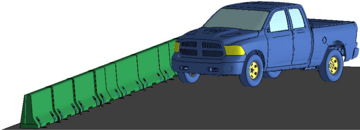
**Figure 2.9. *MASH* Test 3-11 Simulation Setup for the Originally Proposed Barrier Design.**
