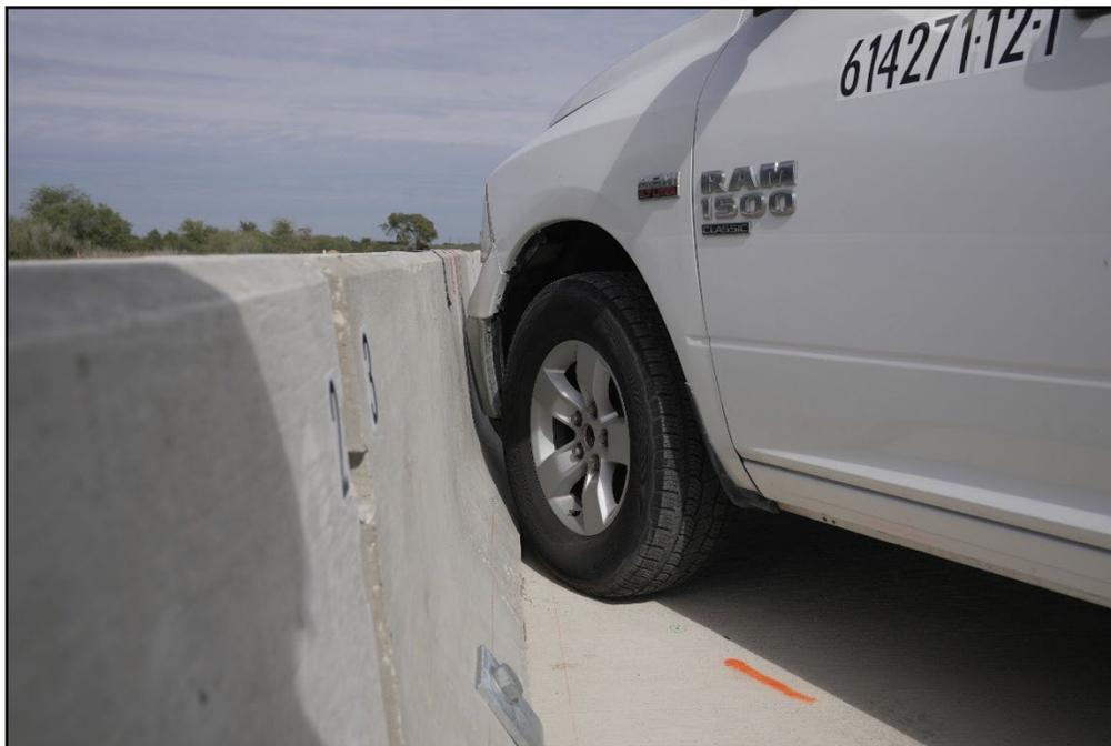
**Figure 7.2. Maryland F-Type Temporary Barrier and Test Vehicle Impact Location for Test 614271-12-1.**
