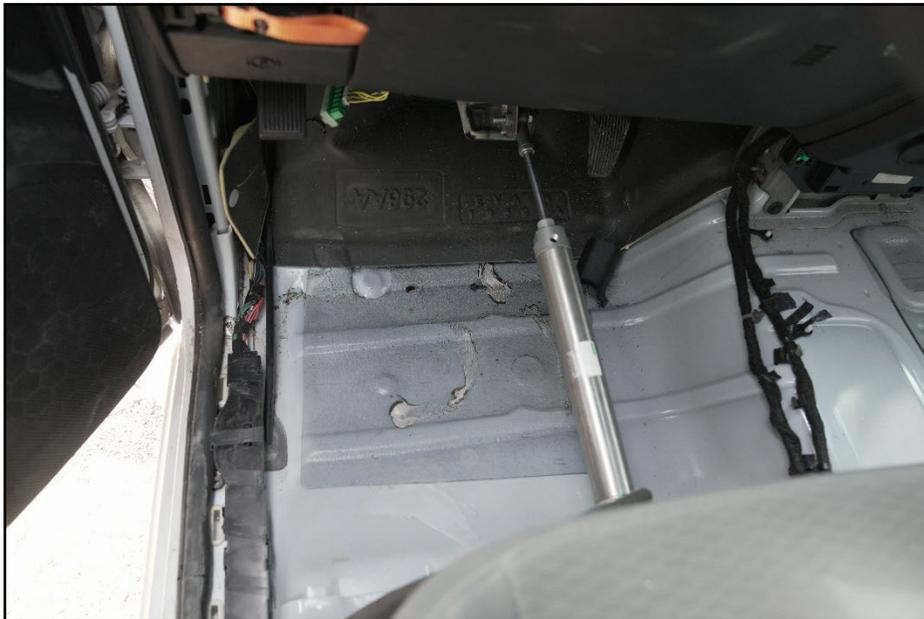
**Figure 7.10. Interior of Test Vehicle on Impact Side after Test 614271-12-1.**
