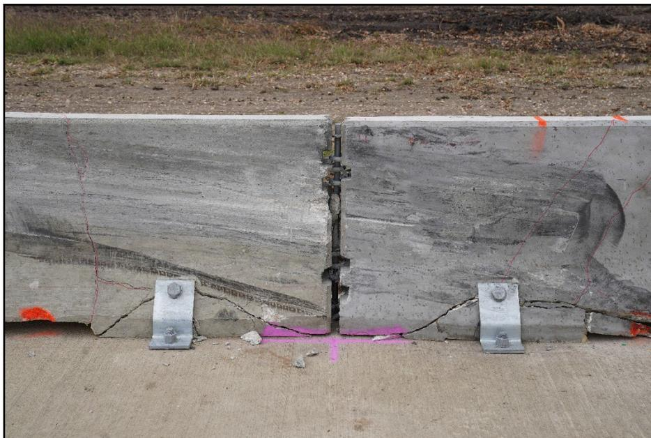
**Figure 6.6. Maryland F-Type Temporary Barrier after Test at the Joint of Barriers 4 and 5 for Test 614271-12-2.**
