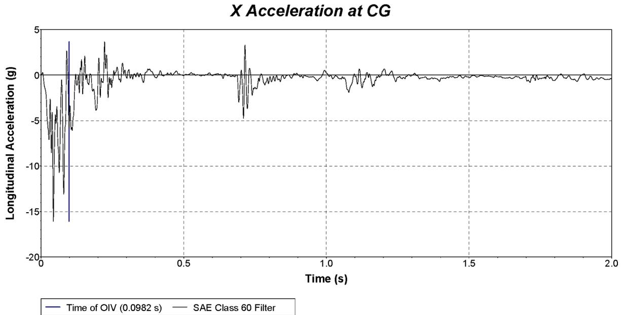
**Figure D.8. Vehicle Longitudinal Accelerometer Trace for Test No. 614271-12-1 (Accelerometer Located at Center of Gravity).**
