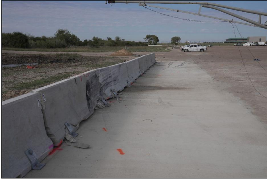
**Figure 7.5. Maryland F-Type Temporary Barrier after Test at Impact Location for Test 614271-12-1.**
