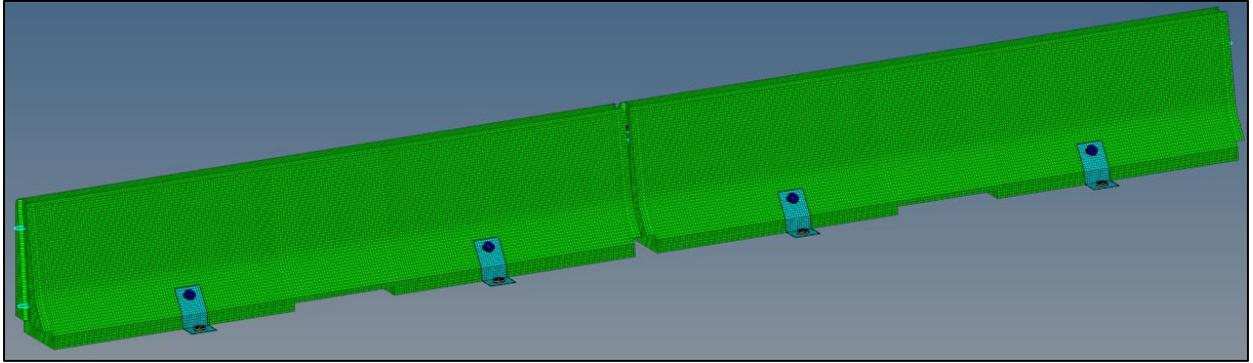
**Figure 2.4. FE Model of Concrete Barrier Segments.**
