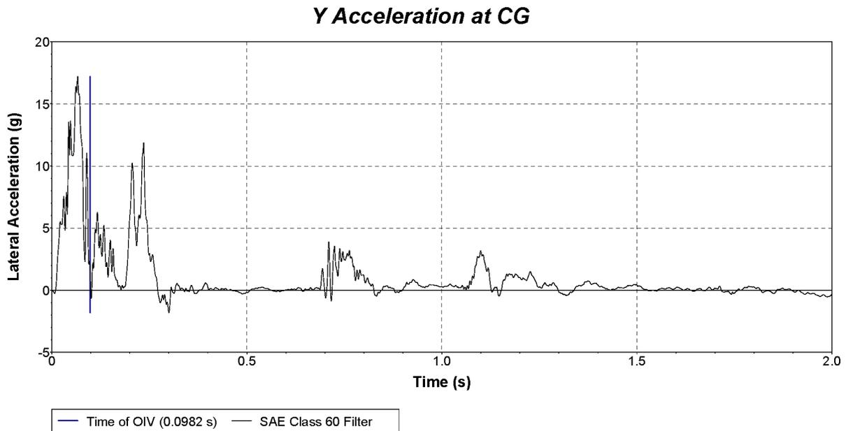
**Figure D.9. Vehicle Lateral Accelerometer Trace for Test No. 614271-12-1 (Accelerometer Located at Center of Gravity).**
