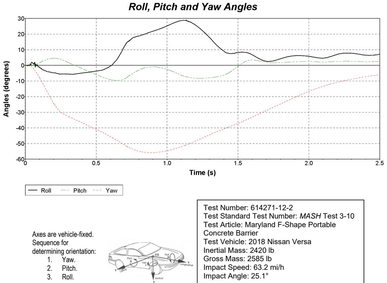
**Figure C.7. Vehicle Angular Displacements for Test No. 614271-12-2.**
