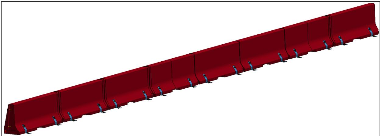
**Figure 2.8. Full System FE Model of Originally Proposed Barrier Design.**
