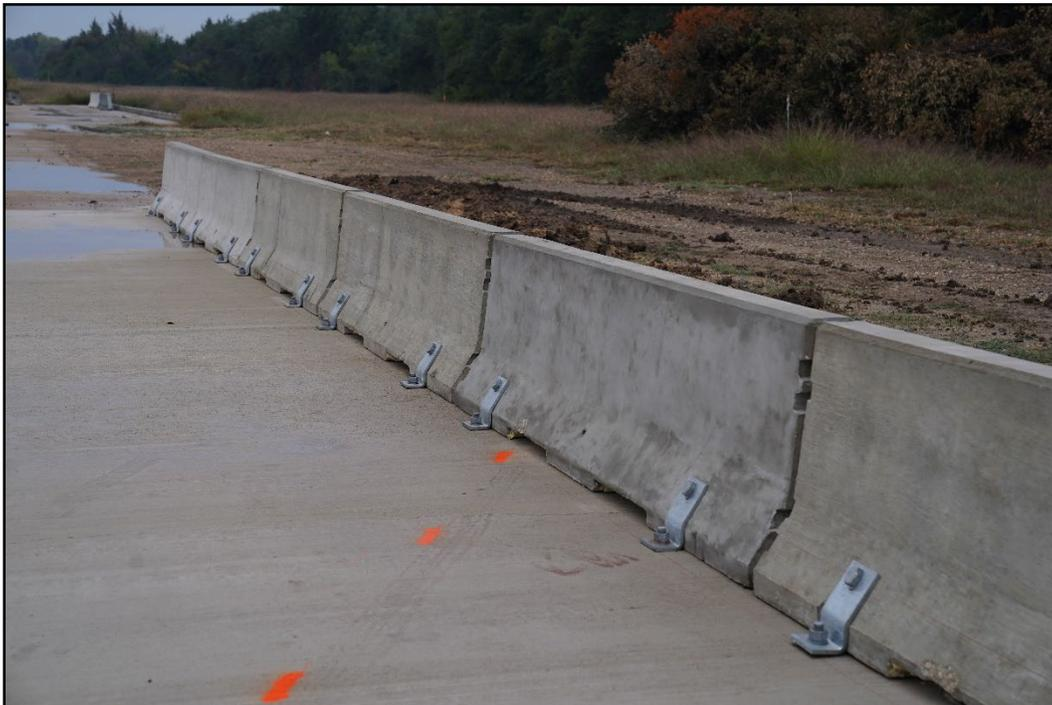
**Figure 3.5. Maryland F-Type Temporary Barrier prior to Testing—Vehicle Tire Trajectory (Orange Line) Aimed at Targeted Barrier-Vehicle Impact Location.**
