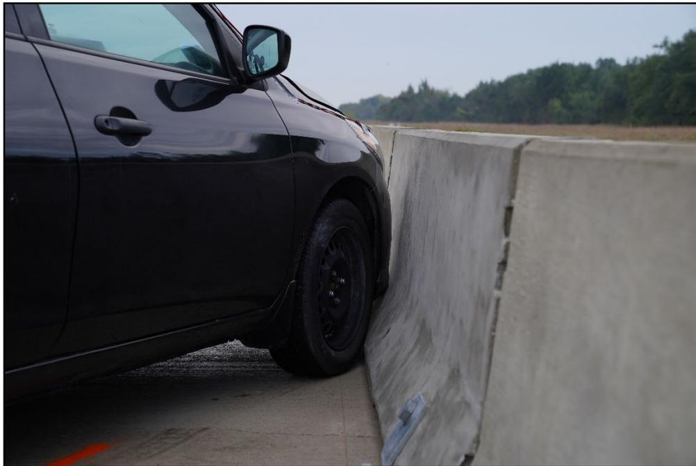
**Figure 6.2. Maryland F-Type Temporary Barrier and Test Vehicle Impact Location for Test 614271-12-2.**
