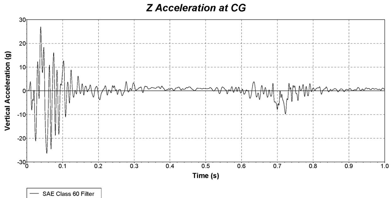
**Figure C.10. Vehicle Vertical Accelerometer Trace for Test No. 614271-12-2 (Accelerometer Located at Center of Gravity).**
