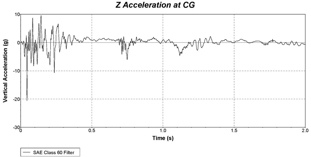
**Figure D.10. Vehicle Vertical Accelerometer Trace for Test No. 614271-12-1
