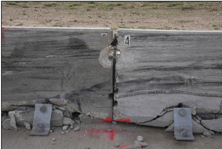
**Figure 7.6. Maryland F-Type Temporary Barrier after Test at the Joint of Barriers 3 and 4 for Test 614271-12-1.**
