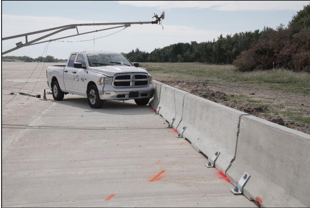
**Figure 7.1. Maryland F-Type Temporary Barrier and Test Vehicle Geometries for Test 614271-12-1.**
