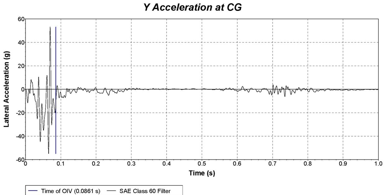
**Figure C.9. Vehicle Lateral Accelerometer Trace for Test No. 614271-12-2
