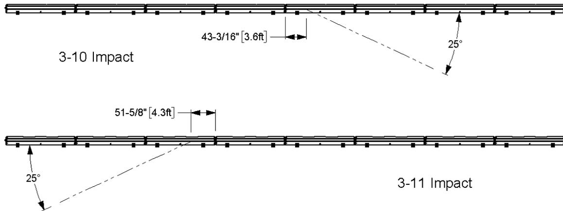
**Figure 4.1. Target CIP for *MASH* TL-3 Tests on Maryland F-Type Temporary Barrier.**
