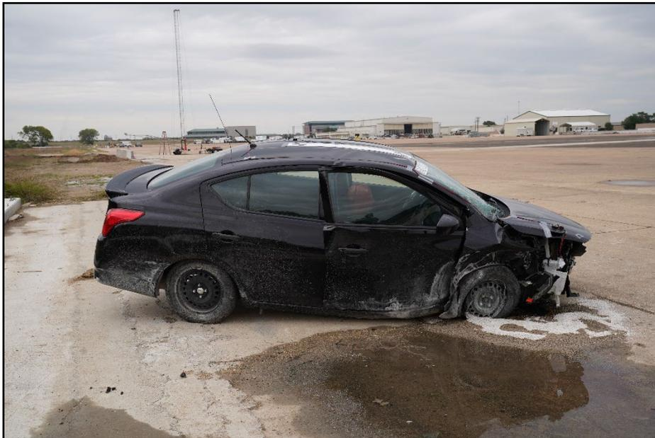
**Figure 6.8. Rear Impact Side of Test Vehicle after Test 614271-12-2.**
