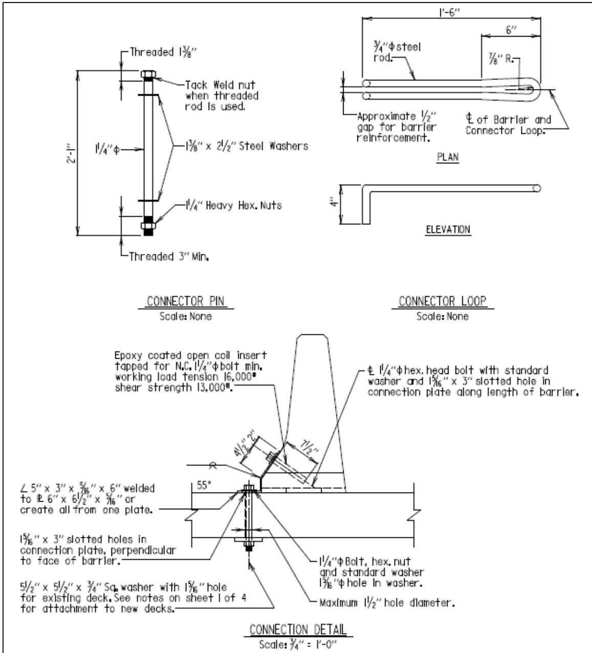
**Figure 2.3. Originally Proposed Design (Not to Be Used for Construction)—Connector Details.**
