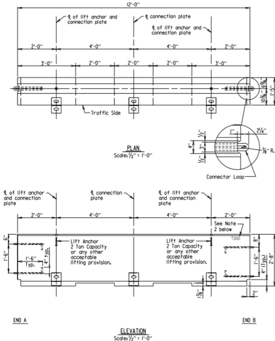
**Figure 2.1. Originally Proposed Design (Not to Be Used for Construction)—General Geometry Details.**
