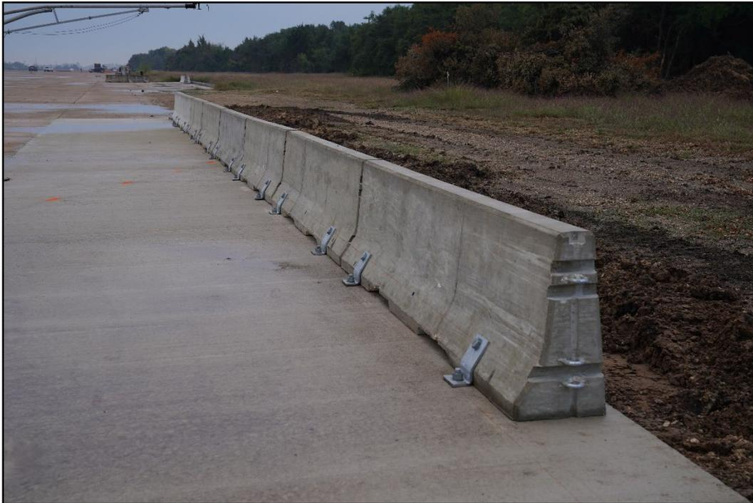
**Figure 3.2. Maryland F-Type Temporary Barrier prior to Testing—Front View of the Installation.**
