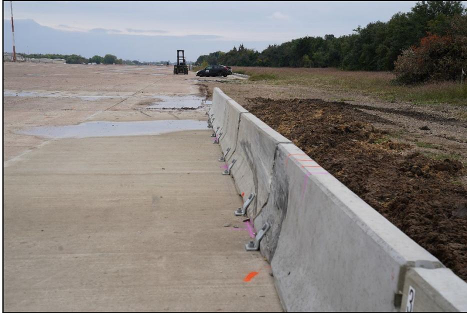
**Figure 6.5. Maryland F-Type Temporary Barrier after Test near Impact Location for Test 614271-12-2.**
