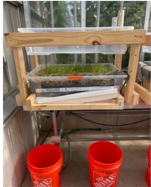
Fig. 1. Example of a constructed Tub with a dual collection system for leachate and runoff
