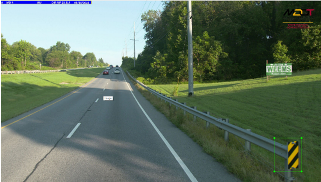
Figure 20. Prepared training images with bounding boxes around objects to be identified
