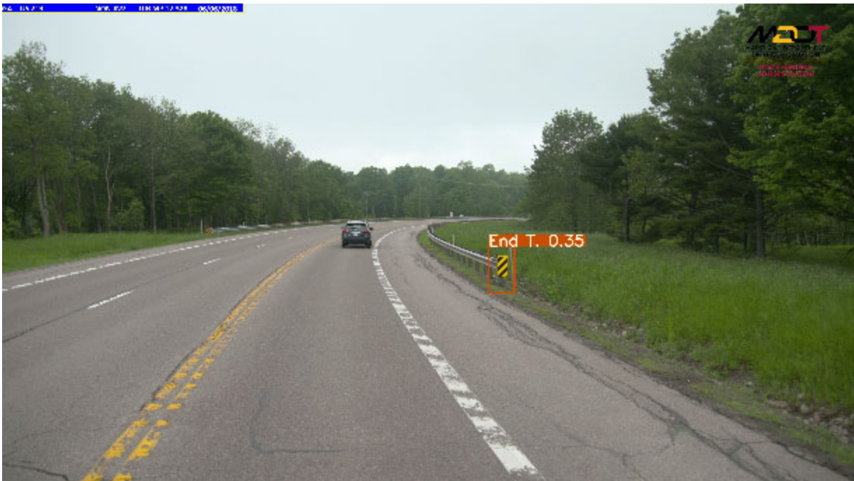
Figure 25. Sample output image with traffic barrier end treatment object identified by YOLO v3 model with tall grass in the background and dashed yellow line marking on the road
