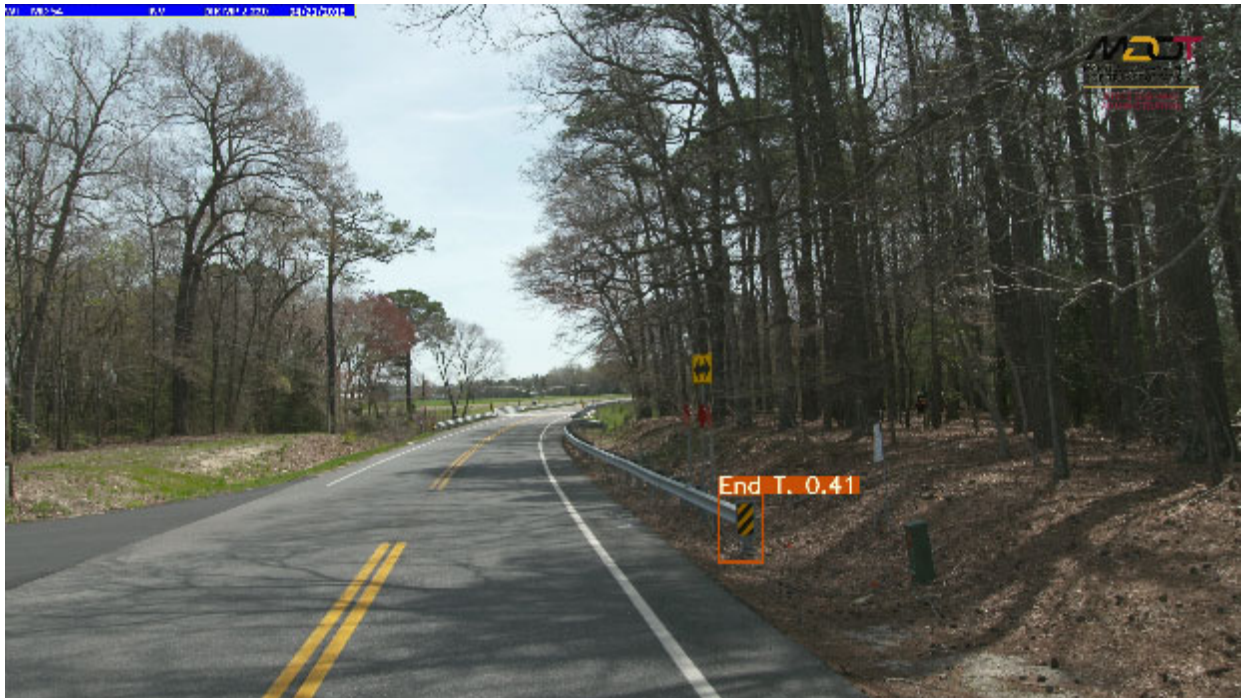
Figure 27. Sample output image with traffic barrier end treatment object identified by YOLO v3 model with medium-scaled traffic barrier end treatment in the picture
