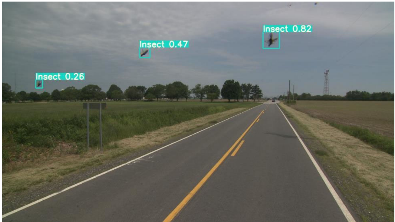
Figure 36. Sample output image with insect objects identified by YOLO v3 model
