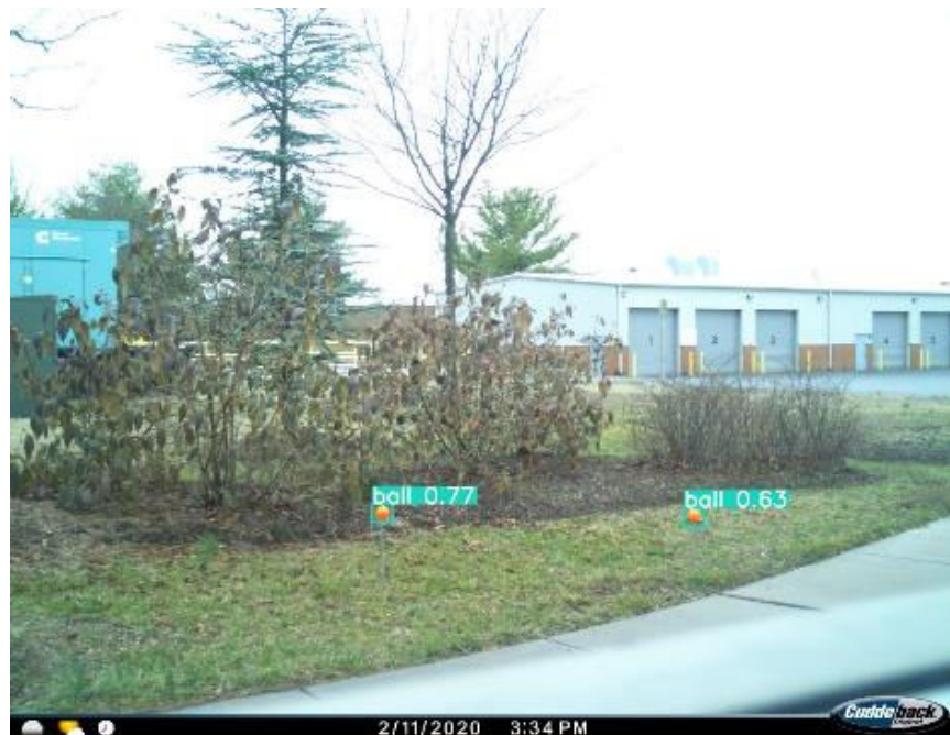
Figure 17. Sample output image with ball objects identified by YOLO v3 model
