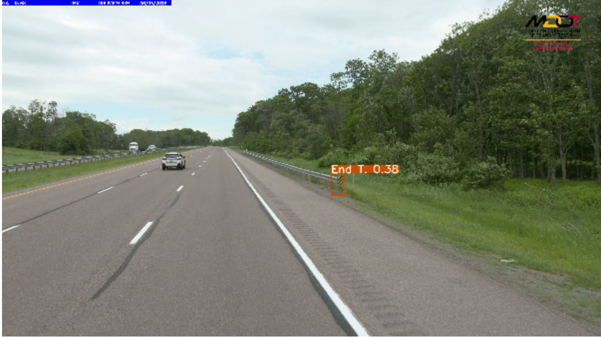
Figure 24. Sample output image with traffic barrier end treatment object identified by YOLO v3 model
