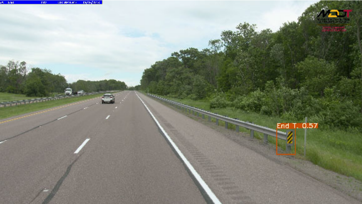
Figure 23. Sample output image with traffic barrier end treatment identified by YOLO v3 model
