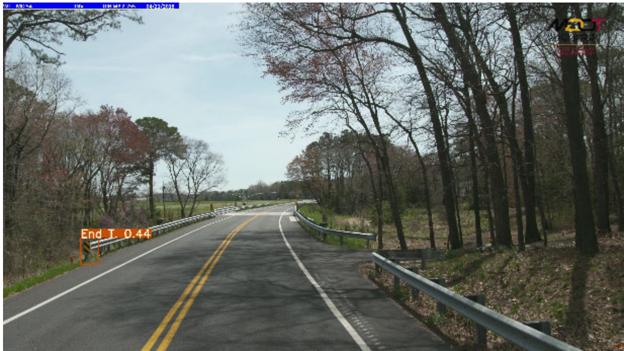
Figure 29. Sample output image with traffic barrier end treatment object identified by YOLO v3 model with traffic barrier end treatment on the left side of the roadway
