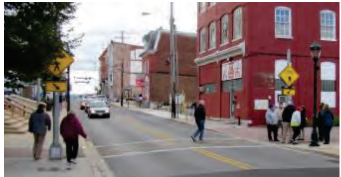
Mid-block Crossing marking and beacons at Antietam Street is a safe accommodation for pedestrians.
