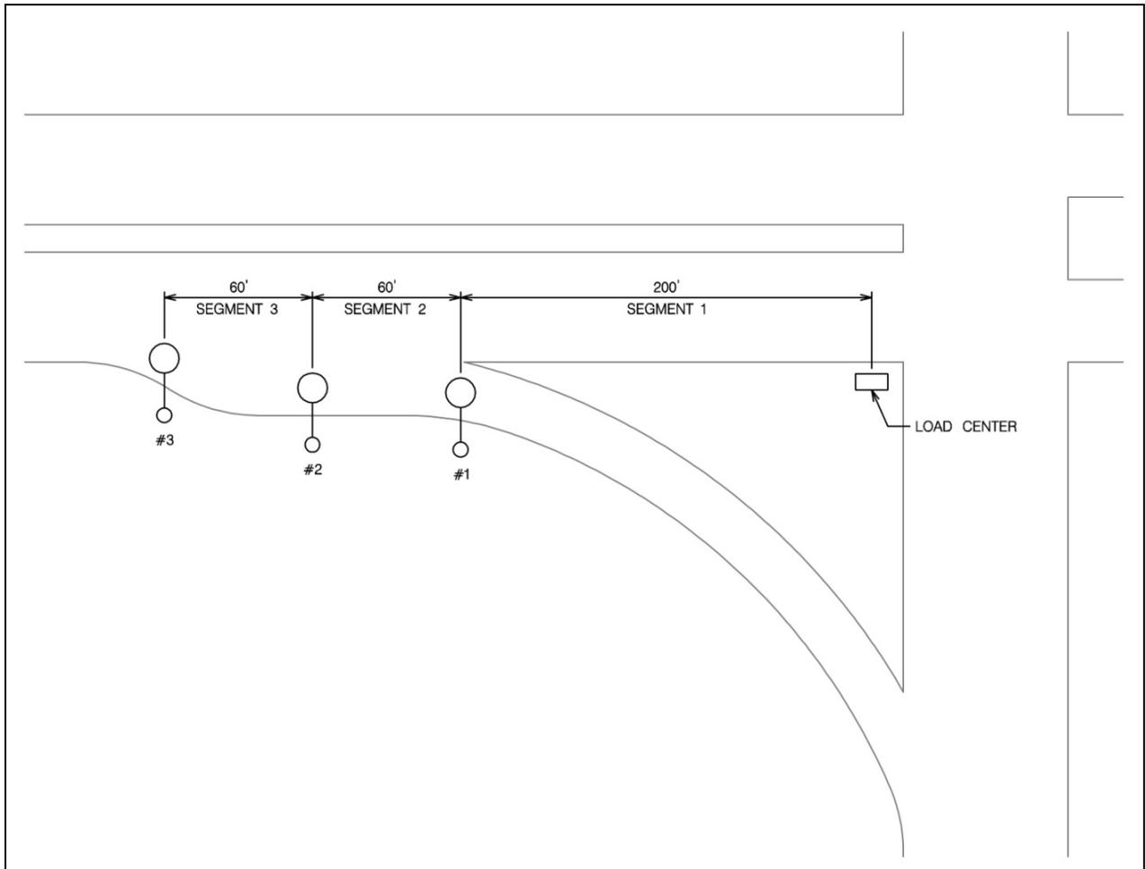
Figure LT.5 - Sample Plan for Voltage Drop Calculation
