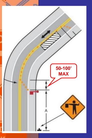
Flagging tapers are used on two-lane, two-way roads where one lane is closed.
