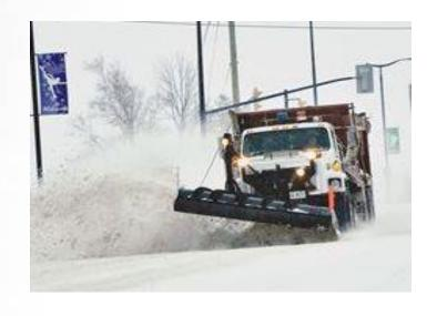
Never plow snow over bridge parapets or jersey barrier walls - that could endanger traffic and/or pedestrians below
