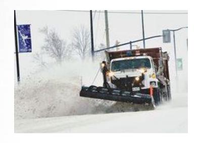
Never plow snow over bridge parapets or jersey barrier walls - that could endanger traffic and/or pedestrians below
