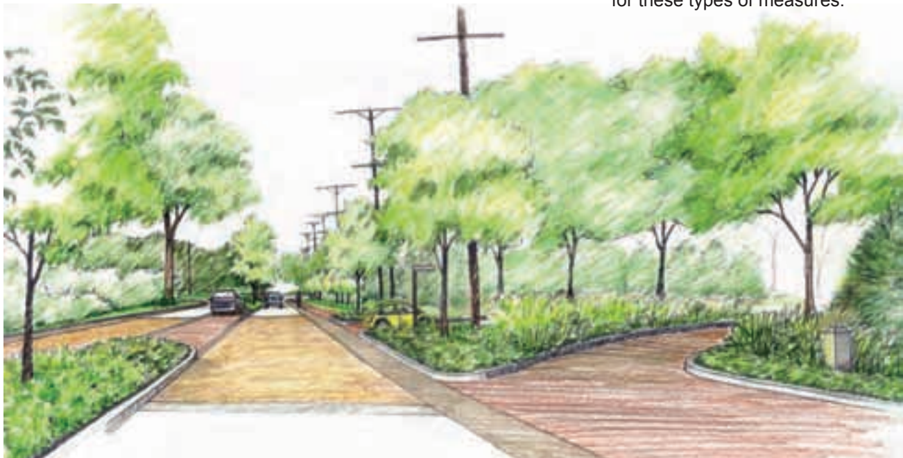
Sketch above illustrates the resulting character that could be achieved for the entrance to a new development planned in the vicinity of Marriottsville Road if context sensitive solutions were applied. Note that the placement of trees closer to the roadway edge can be achieved through the use of barrier curb at intersections (see plan on pages 28-29).
