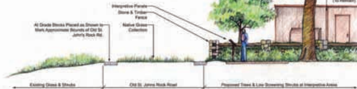
A Cross Section: Interpretive Area at Old St. John's Rock Road scale: 1/4" = 1'-0"
