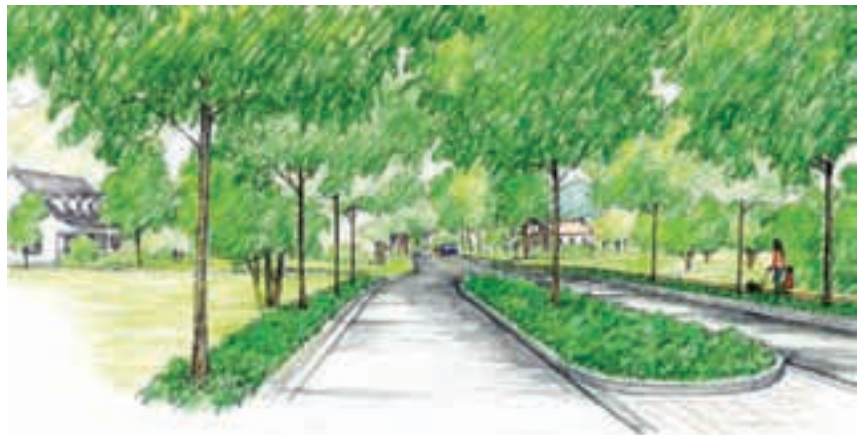
Before and after sketch illustrates proposed use of splitter island to self-enforce desired operating speed within a 25 mph speed zone in Upperville (sketch by Larder/Klein for Route 50 Traffic Calming Project, courtesy of VDOT and H.W. Lochner, Lardner/Klein Landscape Architects, P.C. and Glattig Jackson).
