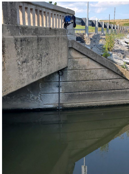
Figure 5. Upstream station (Site ID 01636845) on Little Catoclin Creek near Rosemont, MD, showing the ISCO velocity and area flow module.
