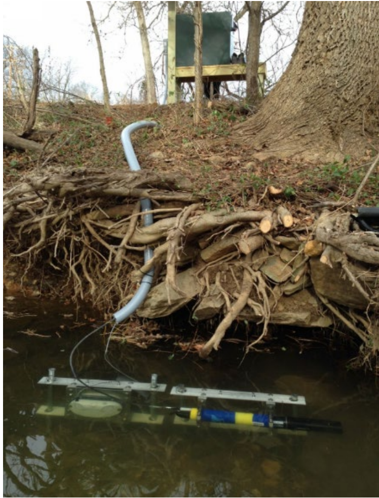
Figure 9. U.S. Geological Survey the downstream station (Site ID 01636846) on Little Catoctin Creek near Rosemont, MD showing the temporary gage station and the discharge and water-quality sonde.
