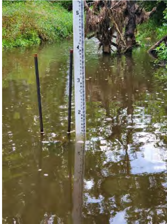
Figure 4. FY23 relocated downstream station (Site ID 01636846) on Little Catoclin Creek near Rosemont, MD. The photo shows the HOBOT logger and stream gage.
