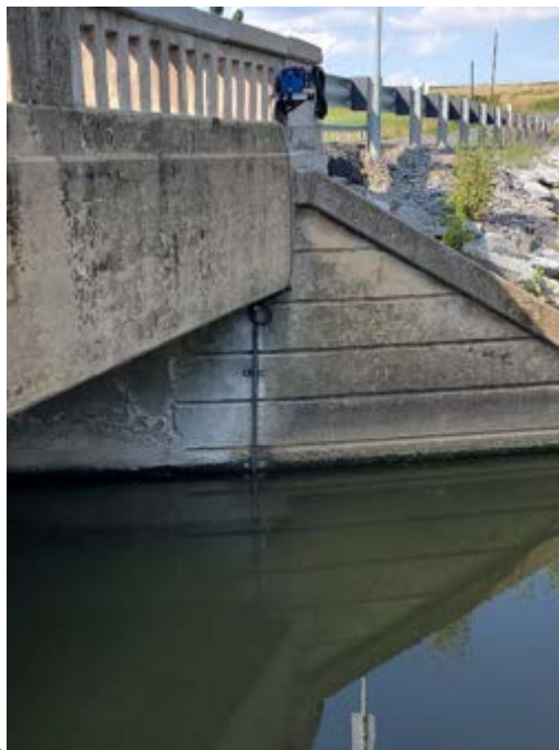
Figure 5. FY22 upstream station (Site ID01636845) on Little Catoctin Creek near Rosemont, MD. The photo shows the ISCO velocity and area flow module.
