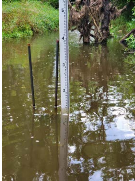
Figure 4. FY22 relocated downstream station (Site ID 01636846) on Little Catoctin Creek near Rosemont, MD. The photo shows the HOBO logger and stream gage.
